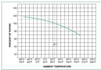
**Note:** Rerating depicted in this curve is in addition to the standard derating of 25% for continuous operation.
