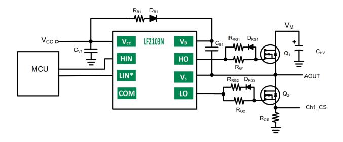
**Figure 4.** Single phase (of four) for Stepper motor driver application using the LF2103N
