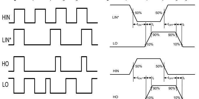
Figure 3. Deadtime Waveform Diagram
