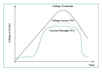
Figure 2: Peak Pulse Power Rating
