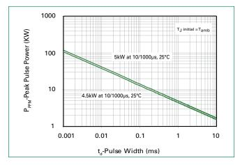
**Figure 3:** Peak Pulse Power Derating Curve
