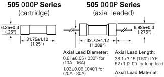
Axial Lead Material: Tin-coated copper
