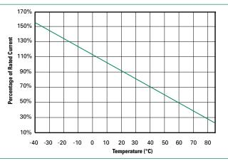
Note: Typical Temperature rerating curve, refer to table for derating data
