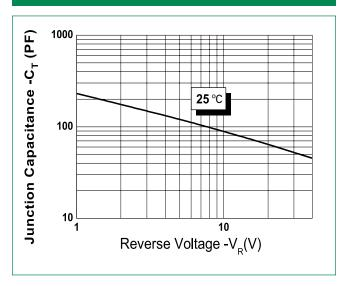
Figure 2: Typical Reverse Characteristics
