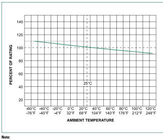
1. Rerating depicted in this curve is in addition to the standard derating of 25% for continuous operation.
