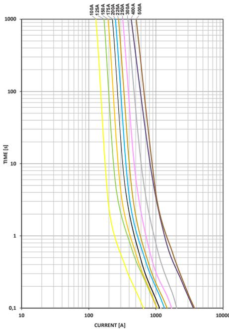
100A-300A:  $F_t=1,25$  (max. operating current:  $0,8 \times I_{rat}$  at 23°C)
