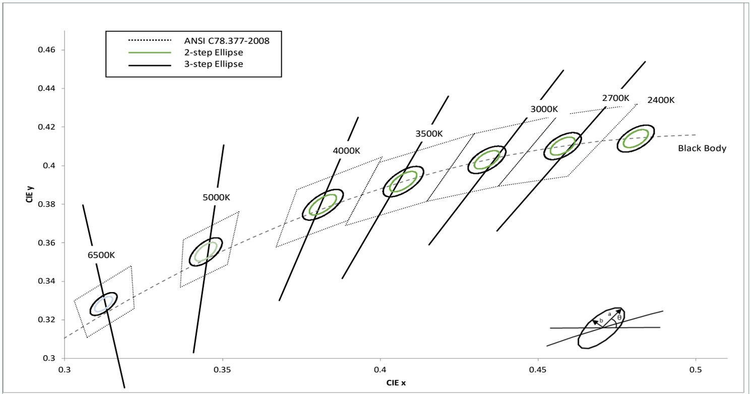
The following tables describe the chromaticity bin center points, the orientation angle for the MacAdam ellipse ( $\theta^\circ$ ), and the maximum radii for the ellipses. The ANSI Bin is provided for reference.
