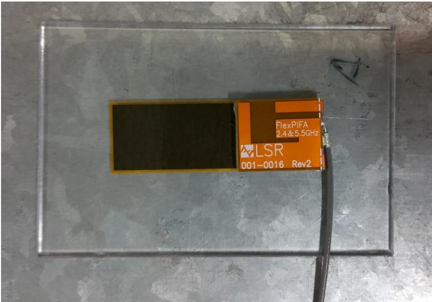
Figure 38: FlexPIFA mounted on metal Surface with 1.5 mm thick polycarbonate spacer
