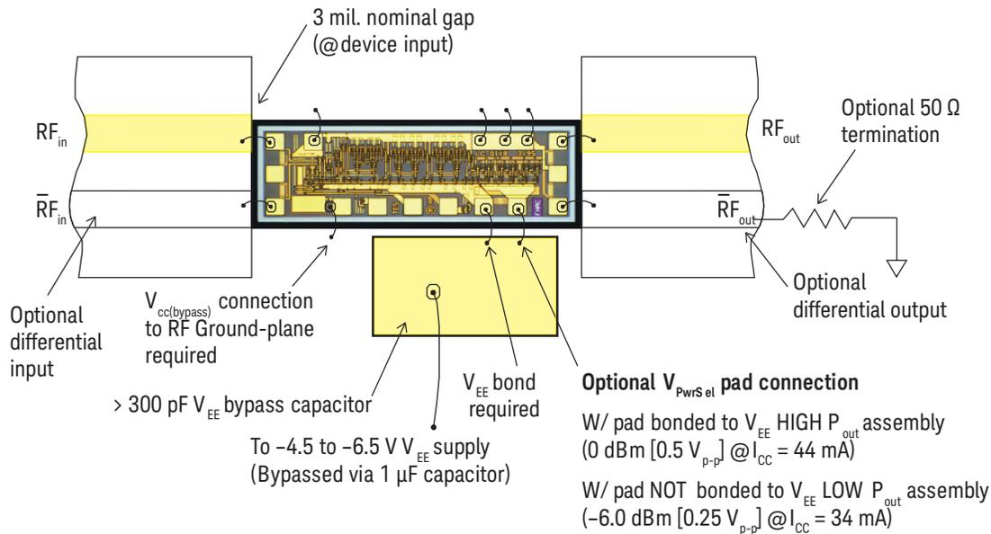
Figure 3. Assembly diagrams
