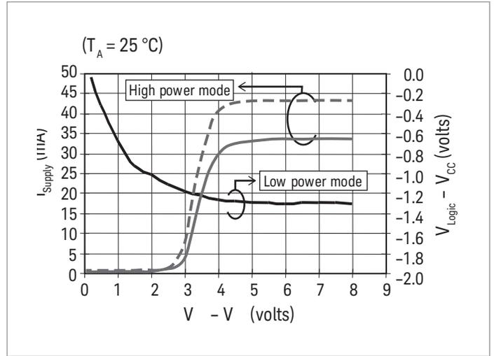
Figure 5. Typical supply current &  $V_{Logic}$  vs. supply voltage
