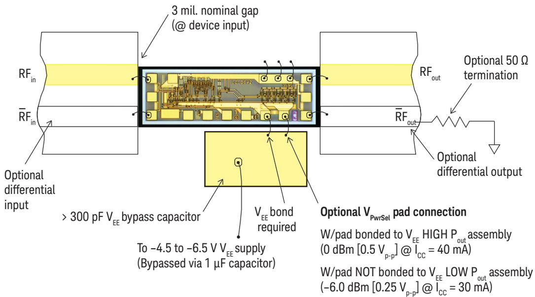
Figure 3. Assembly diagrams
