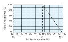
For resistors operated at an ambient temperature of 70°C or higher, the power shall be derated in accordance with the
