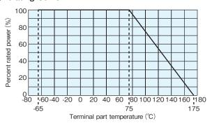
When the terminal part temperature of the resistor exceeds the rated terminal part temperature shown above, the power shall be derated according to the derating curve. \*\*Please refer to "Introduction of the derating curves based on the terminal part temperature" on the
