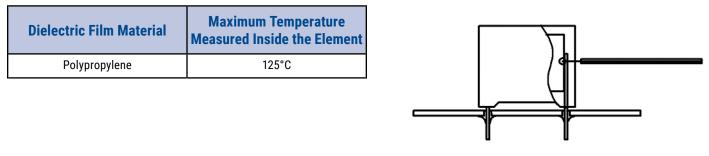
Temperature monitored inside the capacitor.
