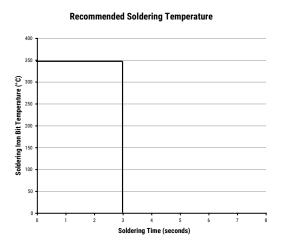
Soldering iron tip temperature should be set at 350°C (+10°C maximum) with the soldering duration not to exceed more than three seconds.
