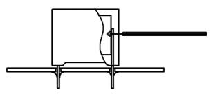
Temperature monitored inside the capacitor.
