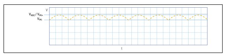
The applied peak-to-peak ripple voltage shall not exceed 0.2 x  $V_{\rm NDC}$ . The peak voltage shall not exceed the rated voltage  $V_{\rm NDC}$ .
