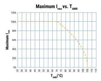
$T_{\text{AMB}}$  is the maximum ambient temperature surrounding the capacitor or hottest contact point (e.g. tracks), whichever is higher, in the worst operation conditions in °C.
