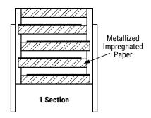
Film Capacitors – AC Line EMI Suppression and RC Networks PMR209, Metallized Impregnated Paper, Class X2, 250 VAC
