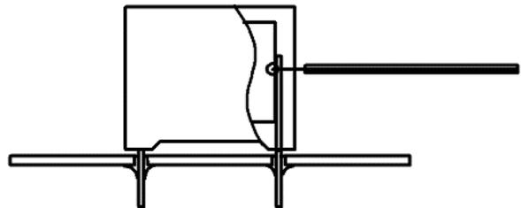
*Temperature monitored inside the capacitor.*
