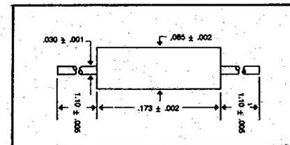
†Standard tolerance of 5, 10, and 20% are available — no suffix is ±20% tolerance. "A" suffix is ±10% tolerance, and "B" suffix is ±5.0% tolerance.
