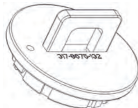
Locking tool for 19-way plug connectors
