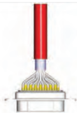
Strip cable 18mm and shape cable to two pigtails
