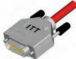
Assemble the other half (screwing force: 100-120 Ncm)
