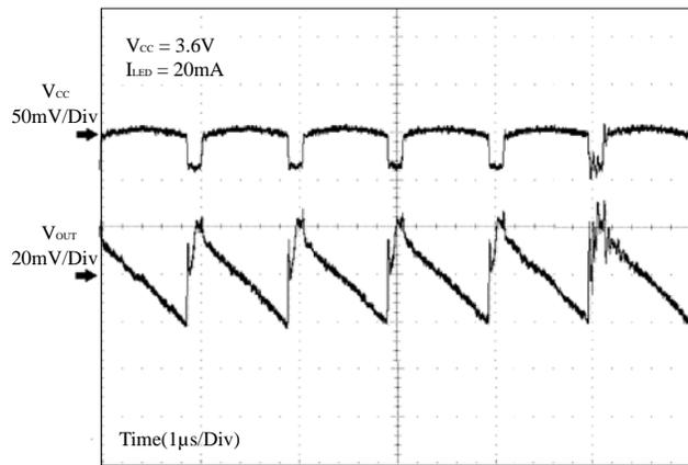
**Figure 9** Ripple Voltage
