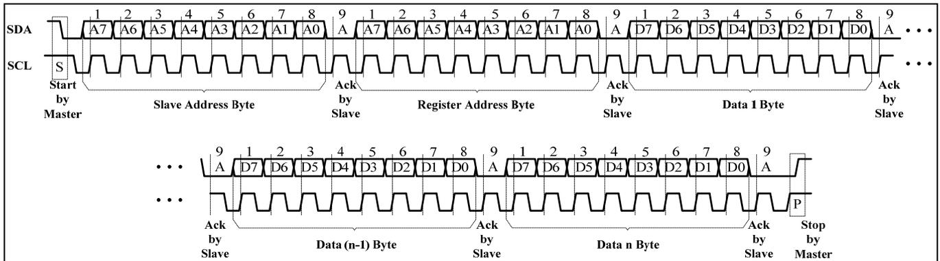
Figure 6 Writing to IS31FL3208A (Automatic Address Increment)
