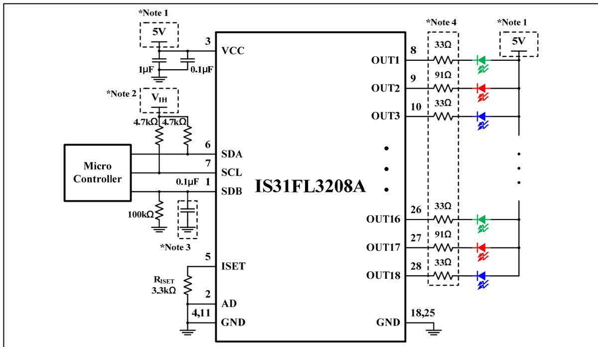
Figure 2 Typical Application Circuit ( $V_{CC}=5V$ )
