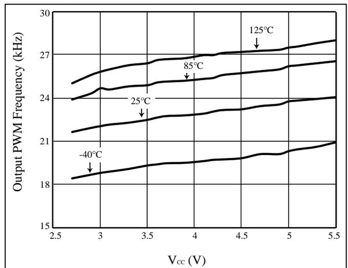
**Figure 9** Output PWM Frequency vs. Vcc
