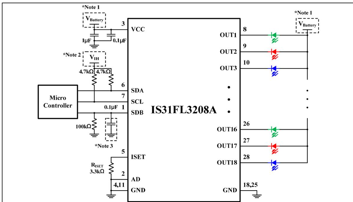
Figure 1 Typical Application Circuit ( $V_{CC}$ = Battery)
