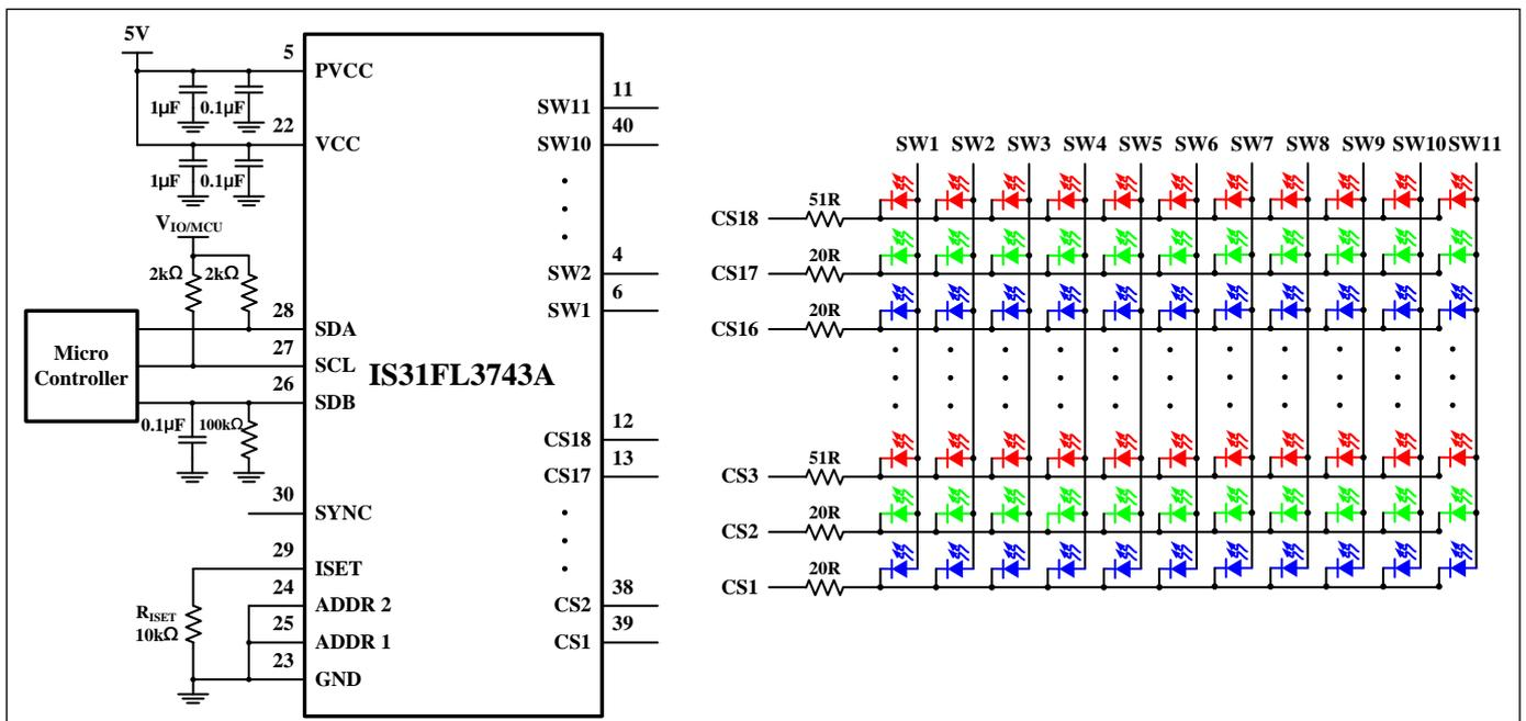
Figure 1 Typical Application Circuit: 66 RGBs
