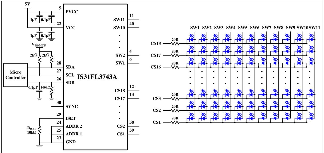
Figure 2 Typical Application Circuit: 198 Mono Color LEDs
