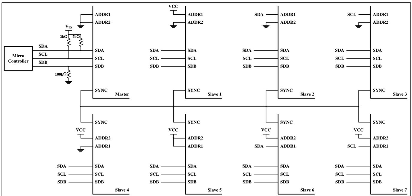
Figure 3 Typical Application Circuit (Eight Parts Synchronization-Work)
