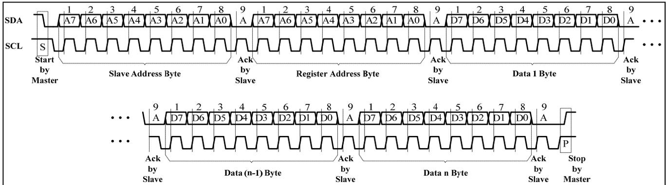
Figure 5 Writing to IS31FL3206 (Automatic Address Increment)
