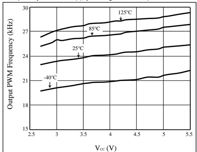
**Figure 8** Output PWM Frequency vs. V<sub>CC</sub>
