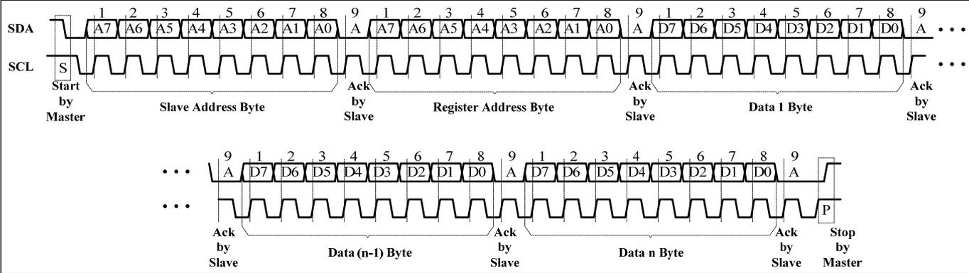
Figure 5 Writing to IS31FL3237 (Automatic Address Increment)
