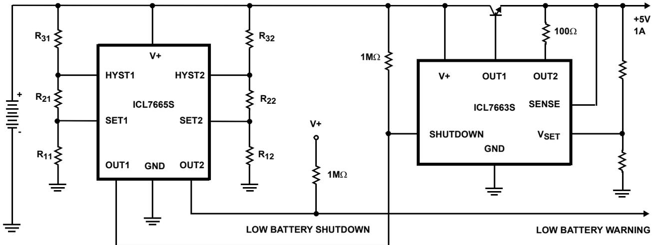
FIGURE 14. LOW BATTERY WARNING AND LOW BATTERY DISCONNECT
