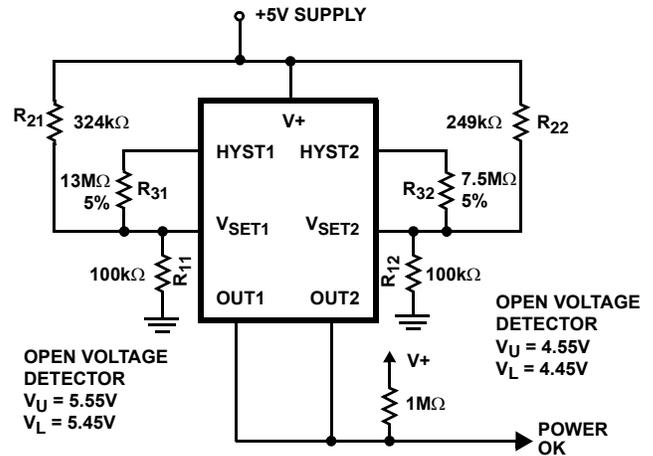
FIGURE 12. FAULT MONITOR FOR A SINGLE SUPPLY
