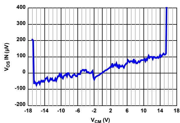
FIGURE 19. V_{OSIN} vs INPUT COMMON MODE VOLTAGE
