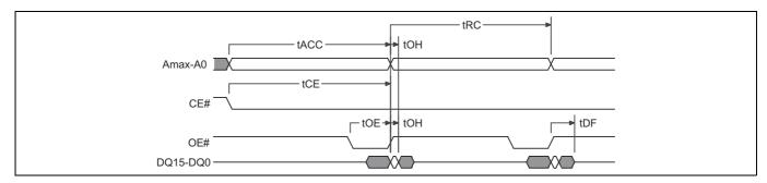
Figure 25 Back to Back Read operation (t<sub>RC</sub>) timing diagram
