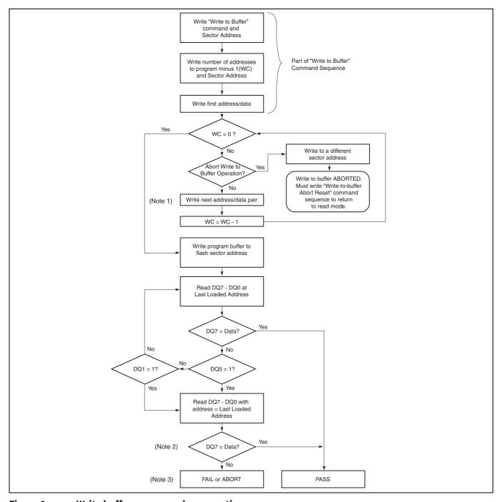
Figure 9 Write buffer programming operation
