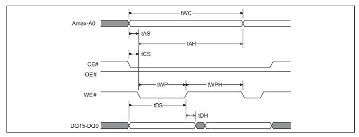
Figure 28 Back to Back (CE# V<sub>IL</sub>) Write operation timing diagram
