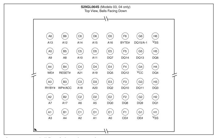
Figure 5 48-ball fine-pitch BGA (VBK 048)
