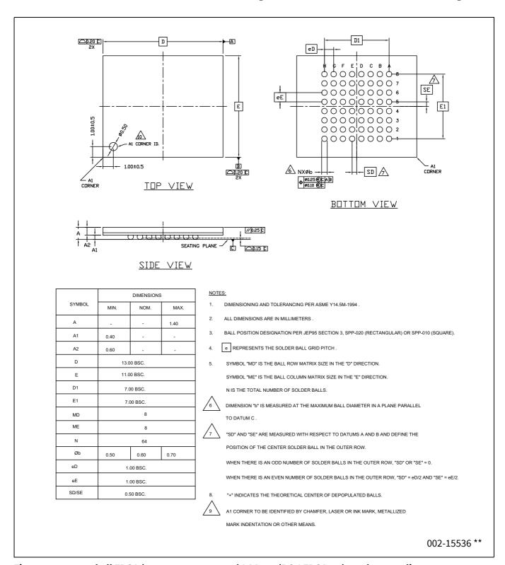
Figure 45 64-ball FBGA (13.0 × 11.0 × 1.4 mm) LAA064 (PG-LFBGA-64), package outline
