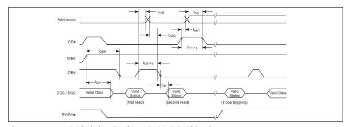
Figure 37 Toggle bit timings (During embedded algorithms)
