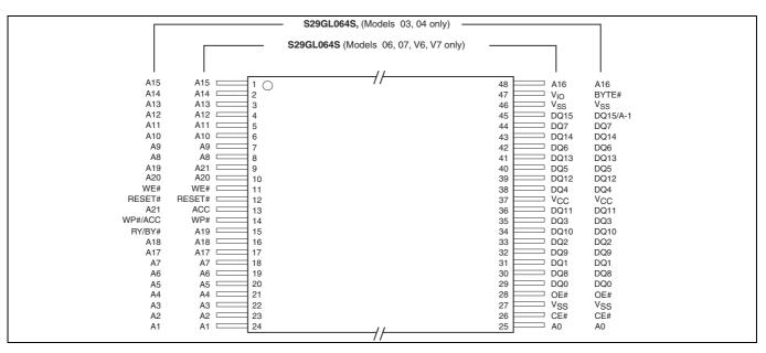
Figure 2 48-lead standard TSOP
