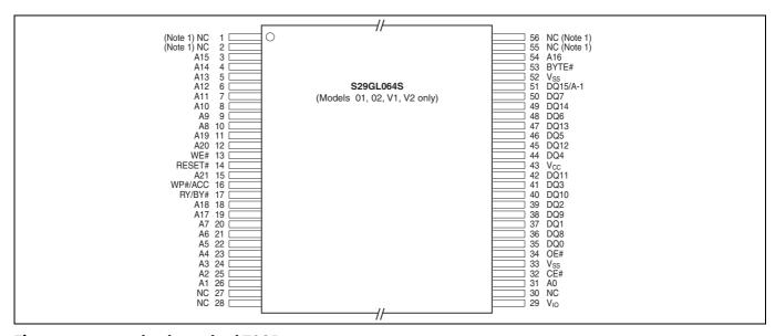
Figure 3 56-lead standard TSOP
