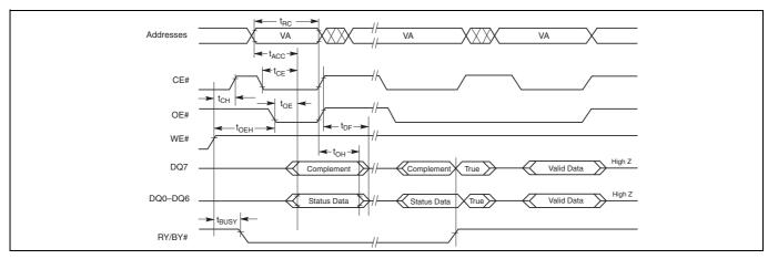
Figure 36 Data# polling timings (During embedded algorithms)
