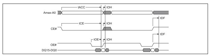
Figure 24 Back to Back Read (t<sub>ACC</sub>) operation timing diagram
