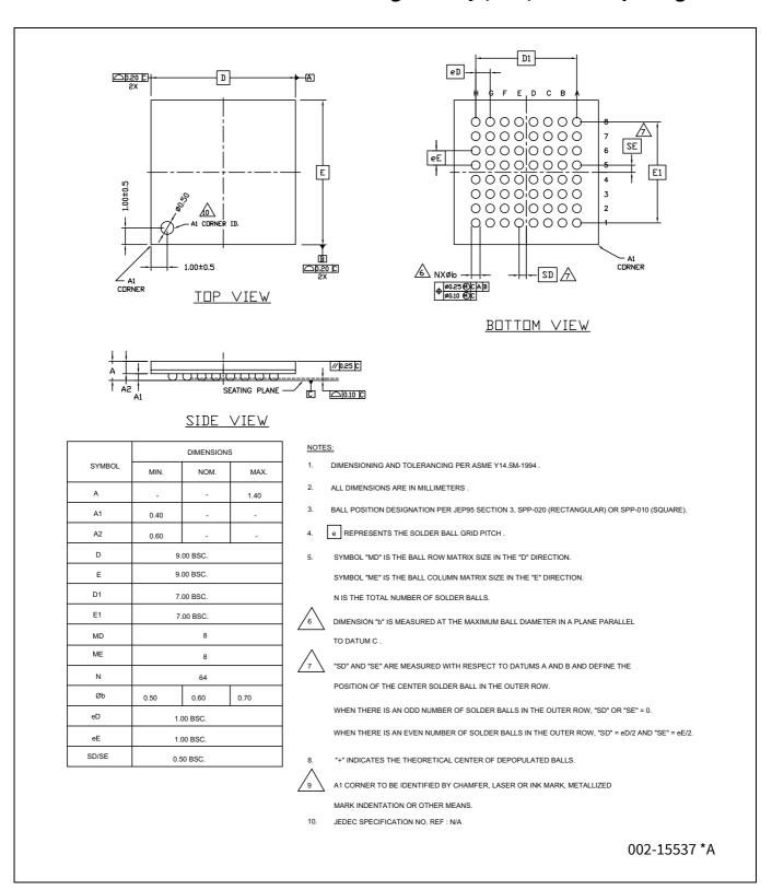
Figure 46 64-ball FBGA (9.0 × 9.0 × 1.4 mm) LAE064 (PG-LFBGA-64), package outline
