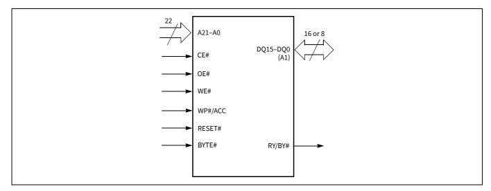
Figure 7 S29GL064S logic symbol (models 03, 04)
