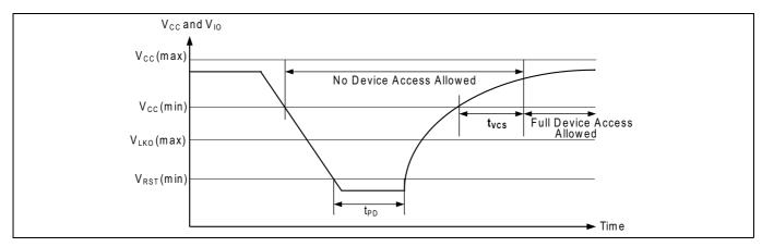
Figure 16 Power-down and voltage drop
