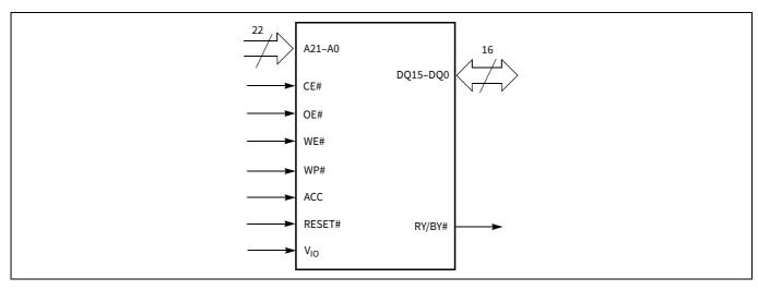
Figure 8 S29GL064S logic symbol (models 06, 07, V6, V7)
