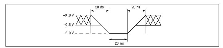
Figure 17 **Maximum negative overshoot waveform**
