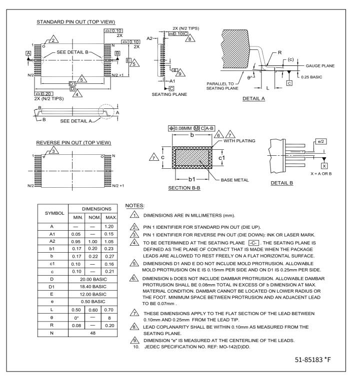
Figure 42 48-lead TSOP (18.4 × 12.0 × 1.2 mm) TS048/TSR048/TS2048/TS4048/ZT48A (PG-TSOP-48), package outline
