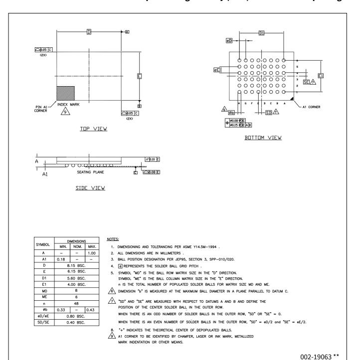
Figure 44 48-ball VFBGA (8.15 × 6.15 × 1.00 mm) VBK048 (PG-VFBGA-56), package outline
