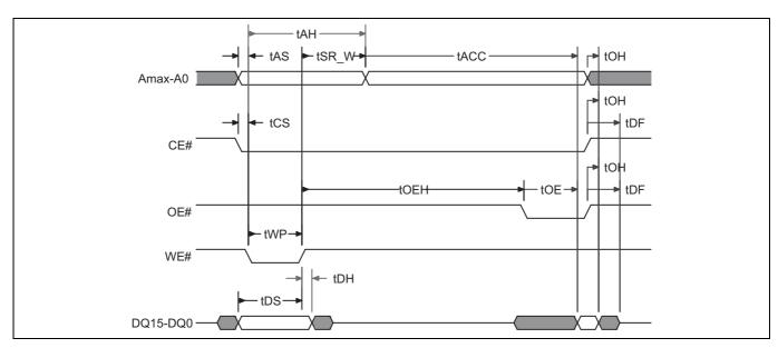
Figure 29 Write to Read  $(t_{ACC})$  operation timing diagram
