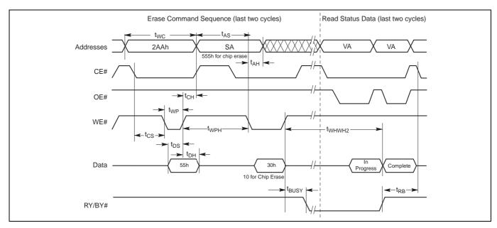
Figure 35 Chip / sector erase operation timings
