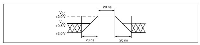
Figure 18 Maximum positive overshoot waveform
