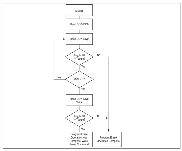
Figure 14 Toggle bit algorithm
