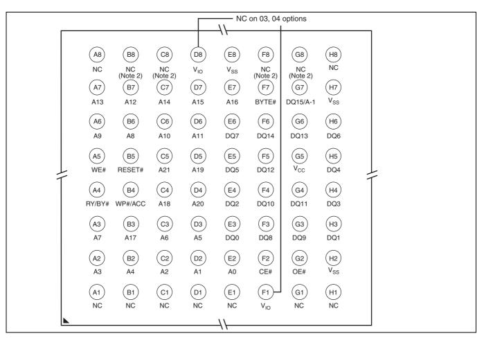
Figure 4 64-ball fortified BGA
