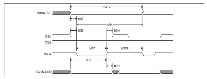
Figure 27 Back to Back Write operation timing diagram
