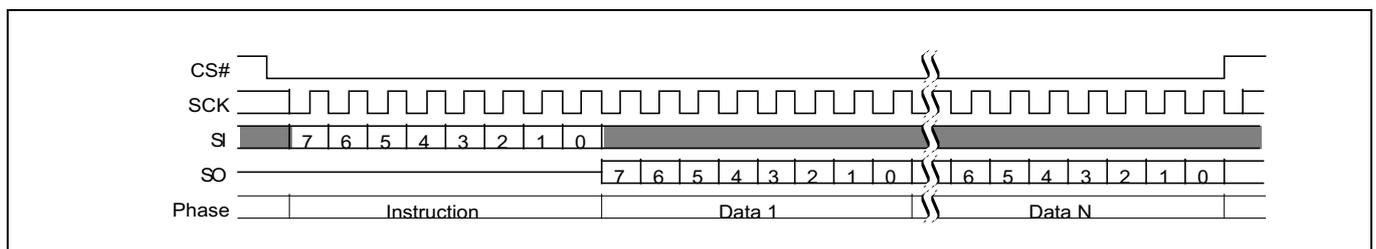
**Figure 44** Read identification (RDID 9Fh) command sequence
