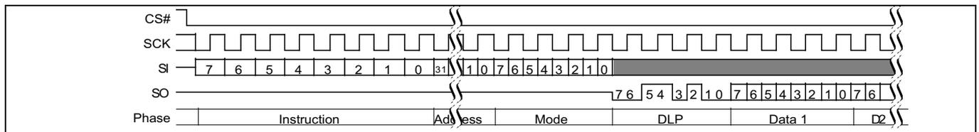
**Figure 84 DDR fast read initial access (4-byte address, 0Eh or 0Dh [ExtAdd=1, EHPLC=01b])<sup>[43]</sup>**
