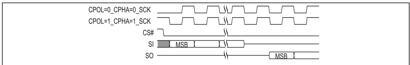
**Figure 5 SPI SDR modes supported**
