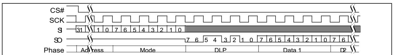
**Figure 85 Continuous DDR fast read subsequent access (4-byte address [ExtAdd=1, EHPLC=01b])<sup>[43]</sup>**
