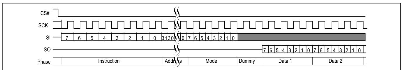
**Figure 16 DDR fast read with EHPLC = 00b**
