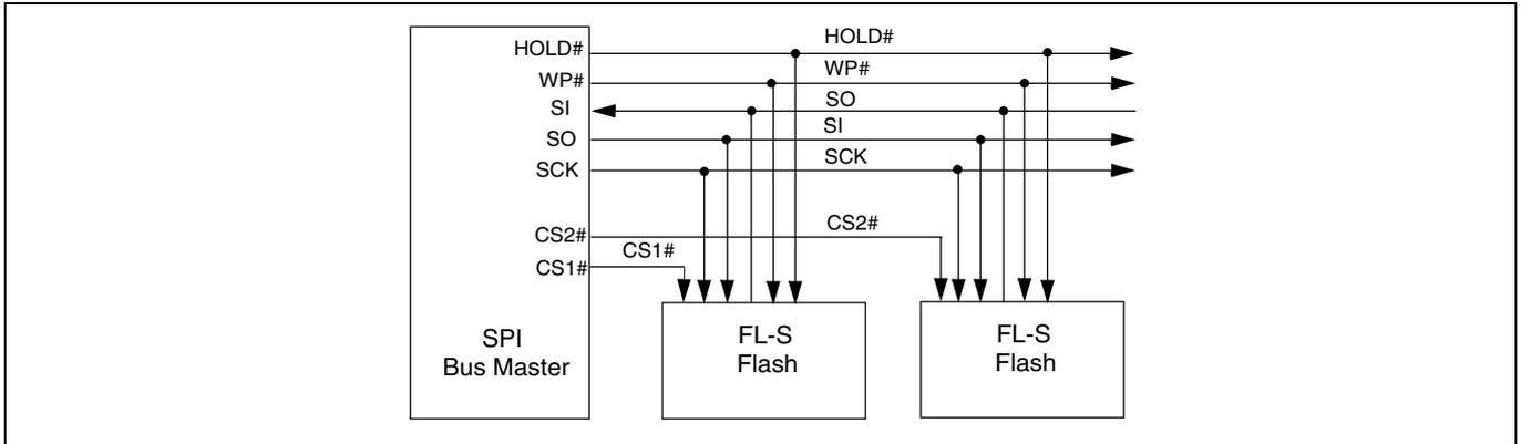
**Figure 2** Bus master and memory devices on the SPI bus — Single bit data path
