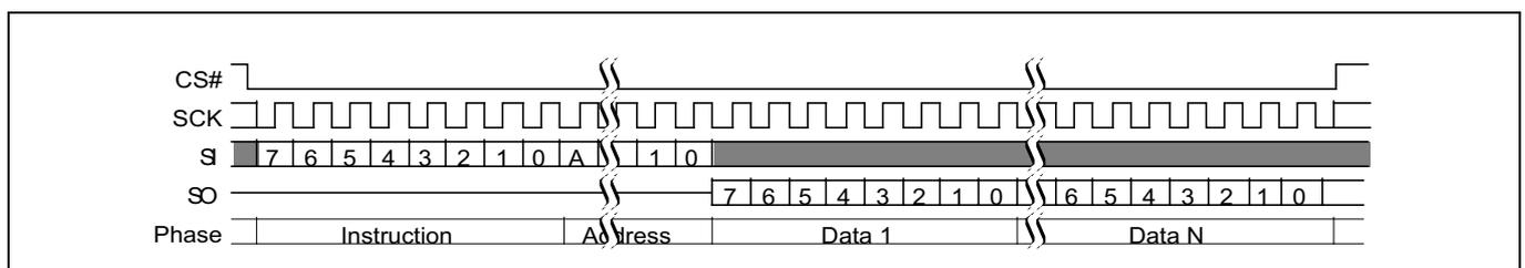
**Figure 68 Fast read command (FAST\_READ 0Bh or 0Ch) sequence without read latency**
