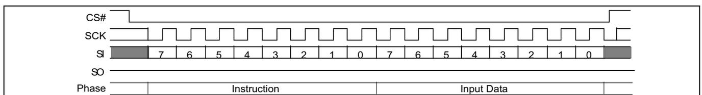
**Figure 63 Program NVDLR (PNVDLR 43h) command sequence**
