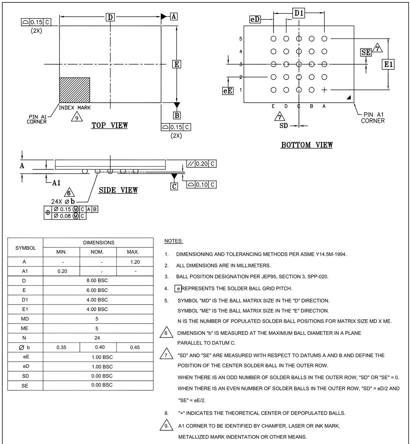
Figure 40 FAB024 — 24-ball BGA (8 x 6 mm) package
