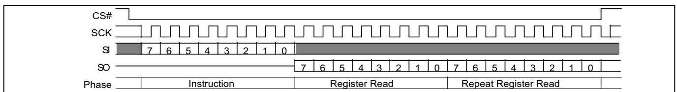
**Figure 50** Read bank register (BRRD 16h) command
