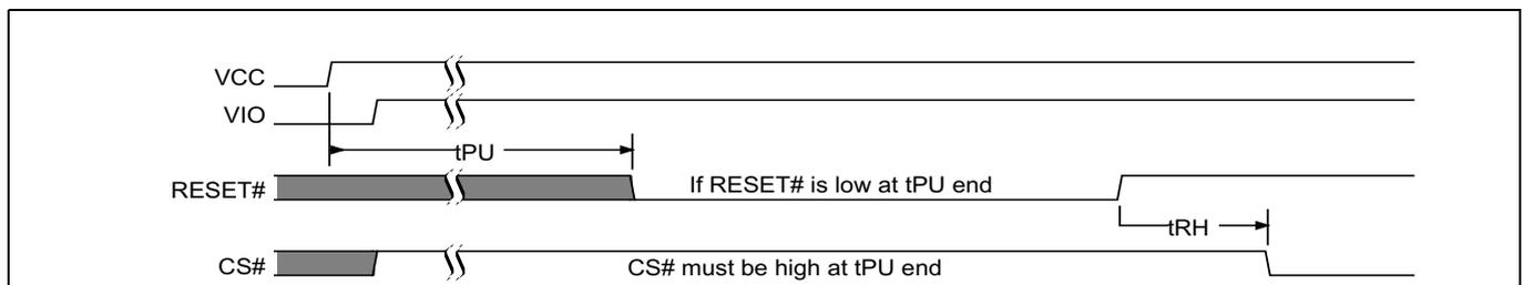
**Figure 26 Reset low at the end of POR**
