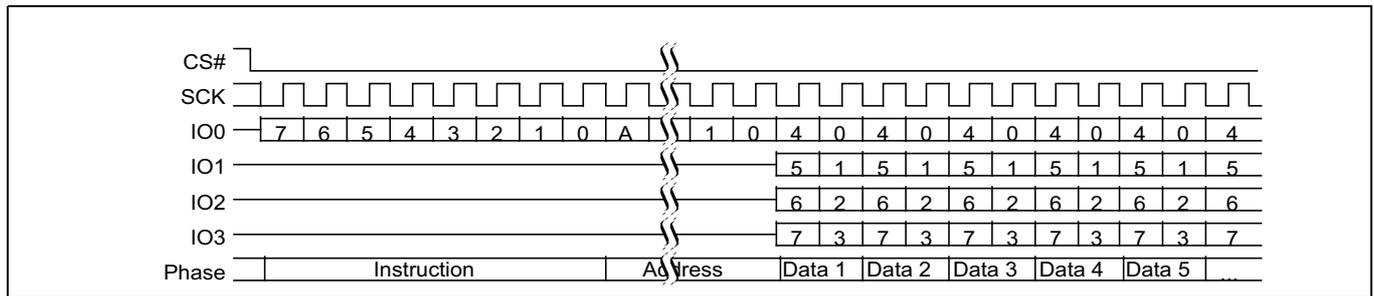
**Figure 73 Quad output read (QOR 6Bh or 4QOR 6Ch) command sequence without read latency**
