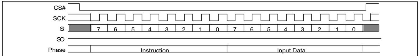
**Figure 51** Bank register write (BRWR 17h) command
