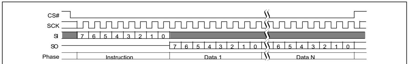
**Figure 113 Password read (PASSRD E7h) command sequence**
