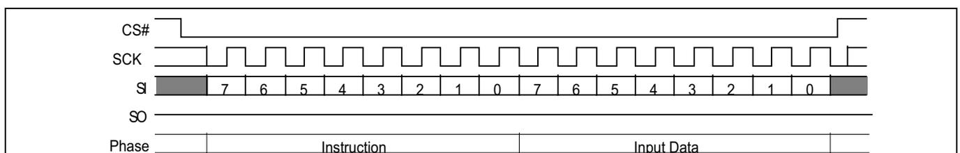
**Figure 8 Single bit wide input command**
