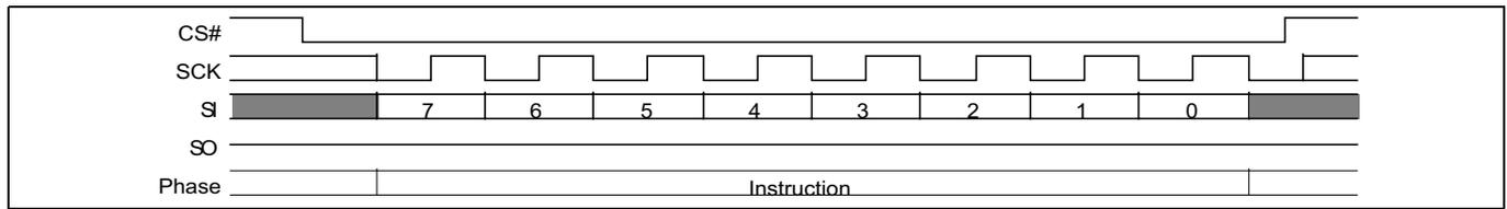
**Figure 117 Mode bit (MBR FFh) reset command sequence**
