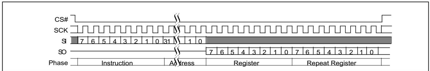
**Figure 108 PPBRD (E2h) command sequence**
