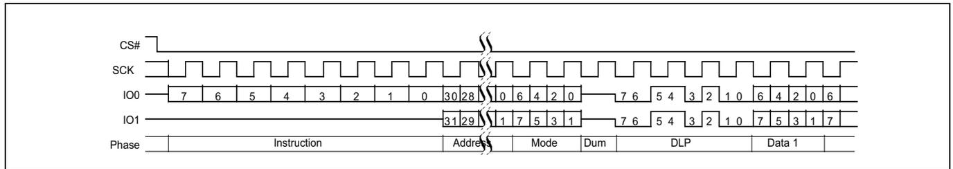
**Figure 17 DDR dual I/O read with EHPLC = 01b and DLP**
