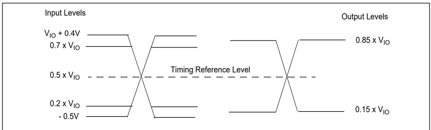
Figure 24 Input, output, and timing reference levels
