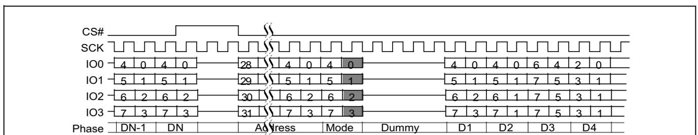
**Figure 81 Continuous quad I/O read command sequence (4-byte address), LC=00b**
