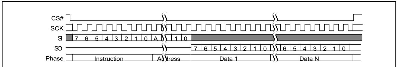
**Figure 66 Read command sequence (READ 03h or 13h)**
