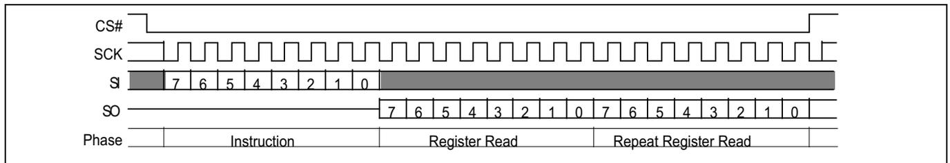
**Figure 111 PPB lock register read command sequence**
