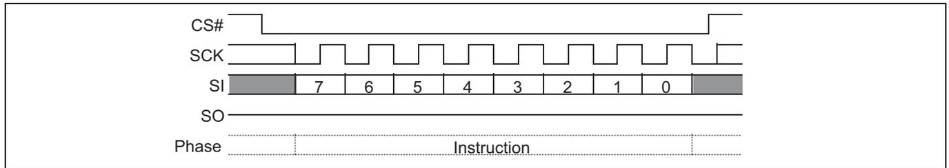
**Figure 97 10.55 Program resume (PGRS 8Ah) command sequence**
