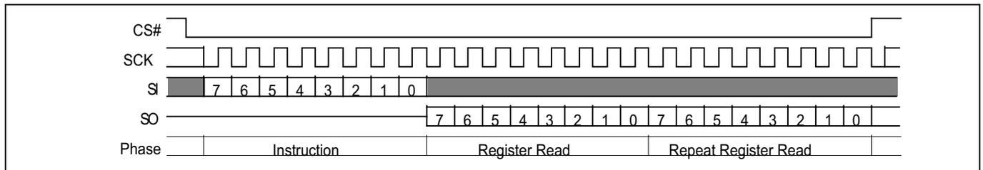
**Figure 49** Read configuration register (RDCR 35h) command sequence
