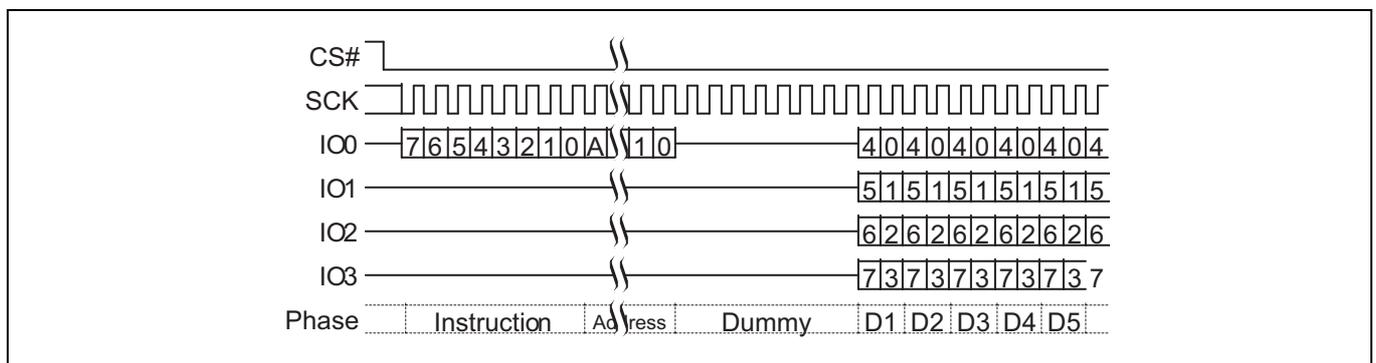
**Figure 72 Quad output read (QOR 6Bh or 4QOR 6Ch) command sequence with read latency**
