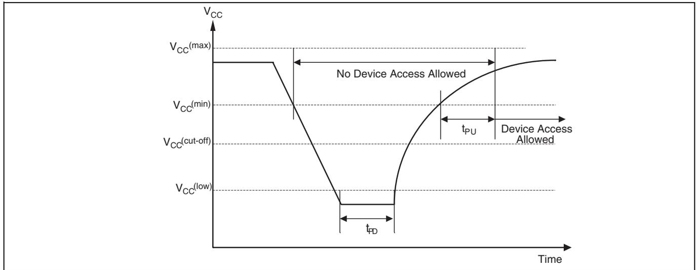
**Figure 22 Power-down and voltage drop**
