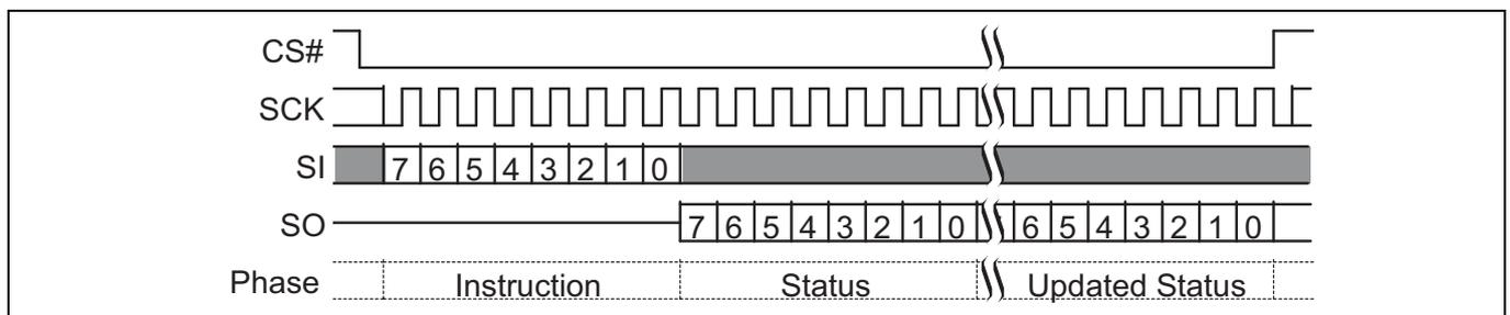
**Figure 47 Read status register-1 (RDSR1 05h) command sequence**
