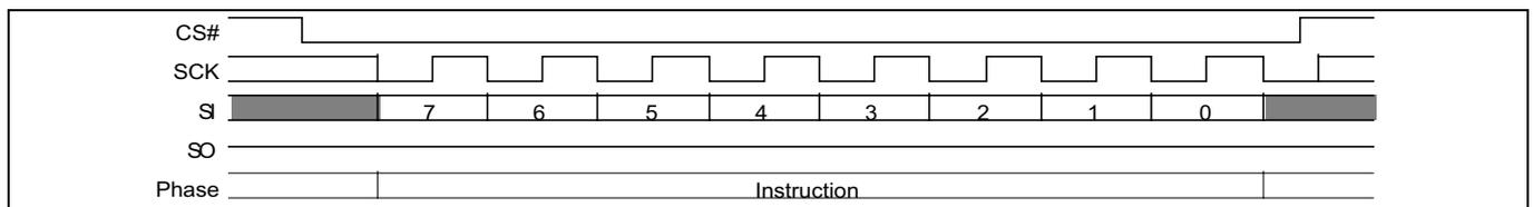
**Figure 116 Software reset (RESET F0h) command sequence**
