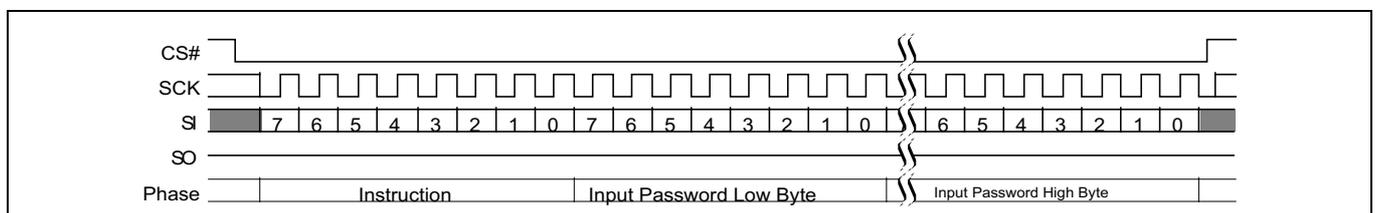
**Figure 114 Password program (PASSP E8h) command sequence**
