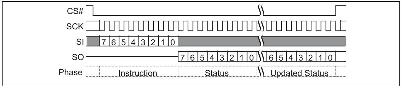
**Figure 48** Read status register-2 (RDSR2 07h) command sequence
