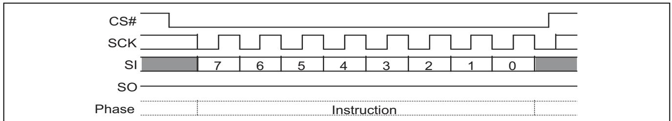
**Figure 55 Write enable (WREN 06h) command sequence**
