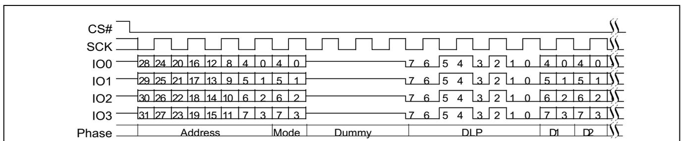
**Figure 93 Continuous DDR quad I/O read subsequent access (4-byte address, EHPLC=01b)<sup>[44]</sup>**
