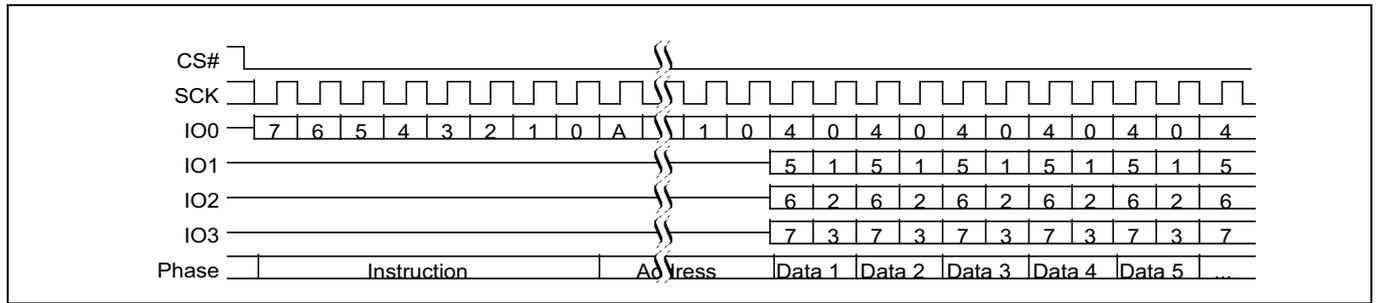
**Figure 95 Quad 512-byte page program command sequence**
