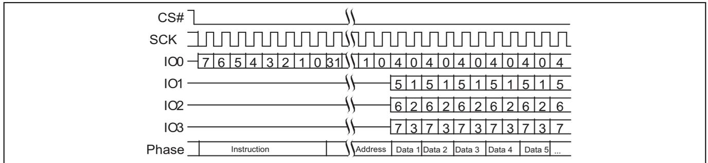
**Figure 13 Quad output command without latency**
