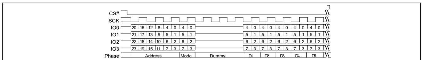
**Figure 91 Continuous DDR quad I/O read subsequent access (3-byte address, HPLC=11b)**
