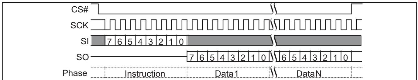
**Figure 61 AutoBoot register read (ABRD 14h) Command**
