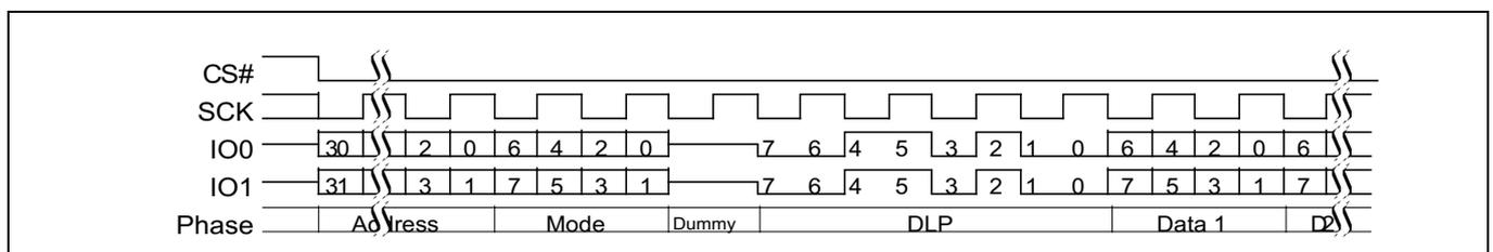
**Figure 88 Continuous DDR dual I/O read subsequent access (4-byte address, EHPLC= 01b)**
