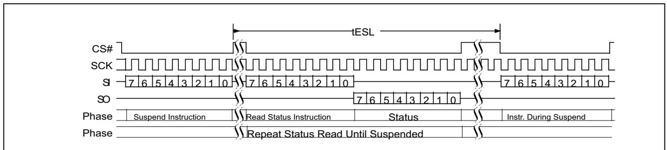
**Figure 100 Erase suspend (ERSP 75h) command sequence**
