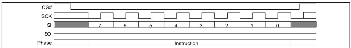
**Figure 112 PPB lock bit write (PLBWR A6h) command sequence**
