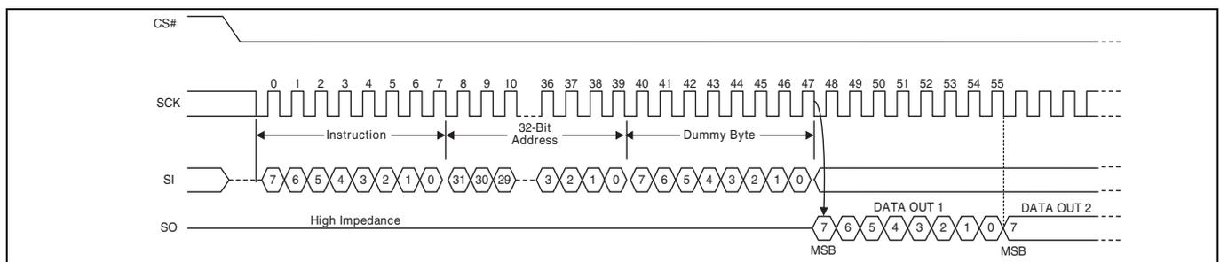
**Figure 58** ECC status register read command sequence
