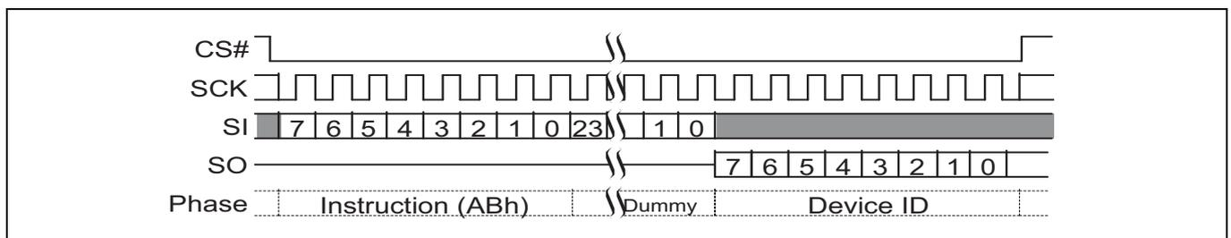
**Figure 45** Read electronic signature (RES ABh) command sequence
