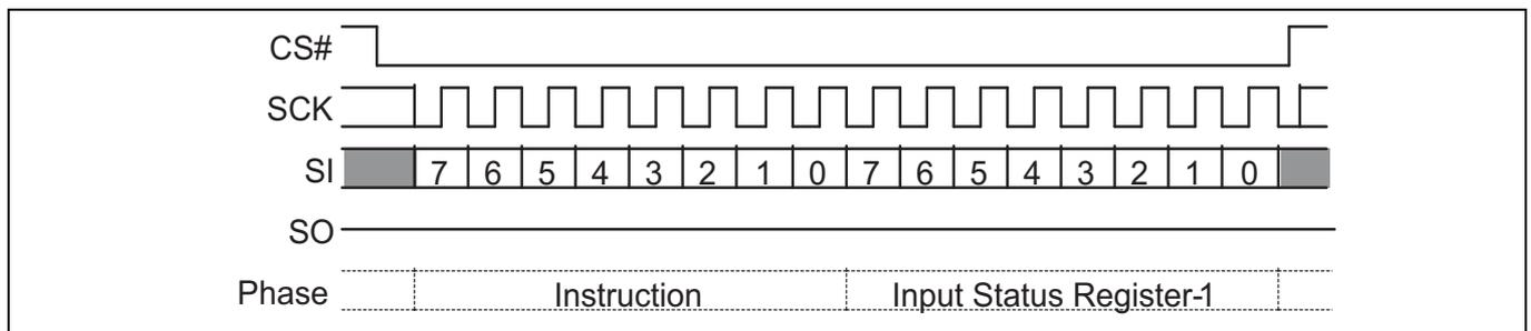
**Figure 53 Write registers (WRR 01h) command sequence – 8 data bits**
