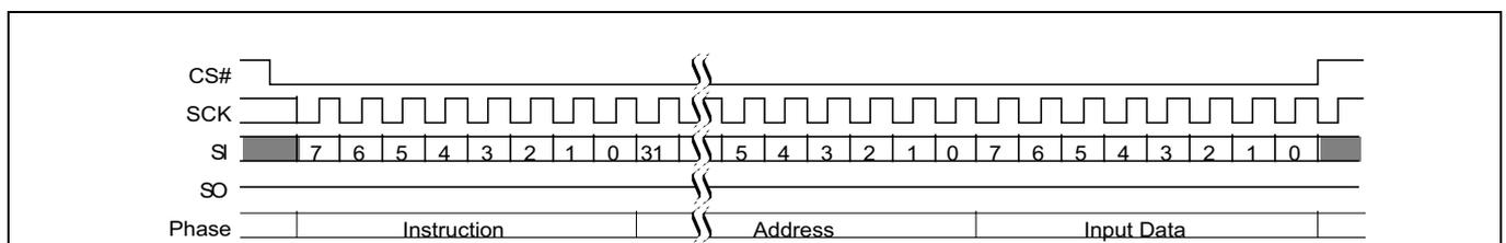
**Figure 107** DYBWR (E1h) command sequence
