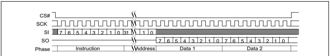
**Figure 10 Single bit wide I/O command without latency**
