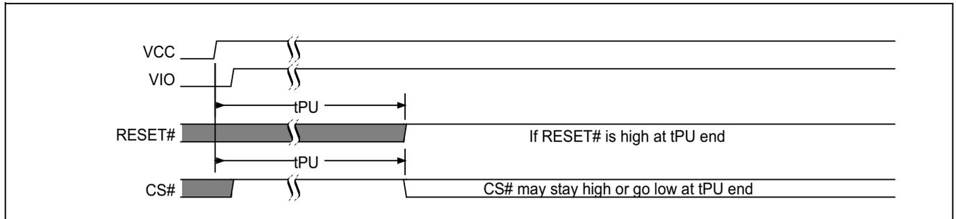
**Figure 27** Reset high at the end of POR
