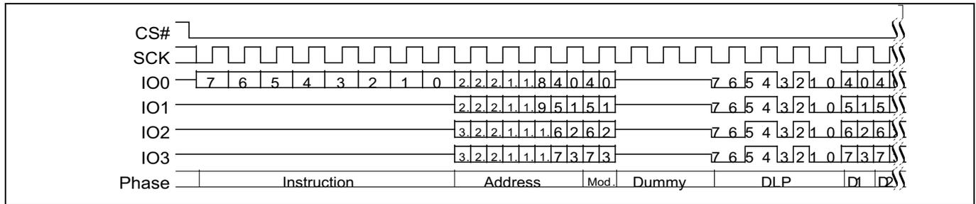
**Figure 92 DDR quad I/O read initial access (4-byte address, EEh or EDh [ExtAdd=1], EHPLC=01b)<sup>[44]</sup>**
