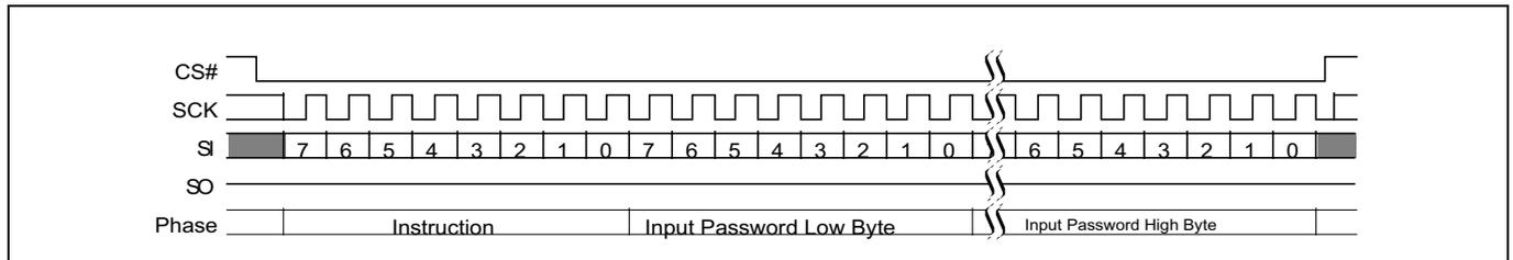
**Figure 115 Password unlock (PASSU E9h) command sequence**
