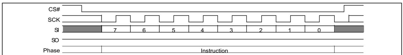
**Figure 56 Write disable (WRDI 04h) command sequence**
