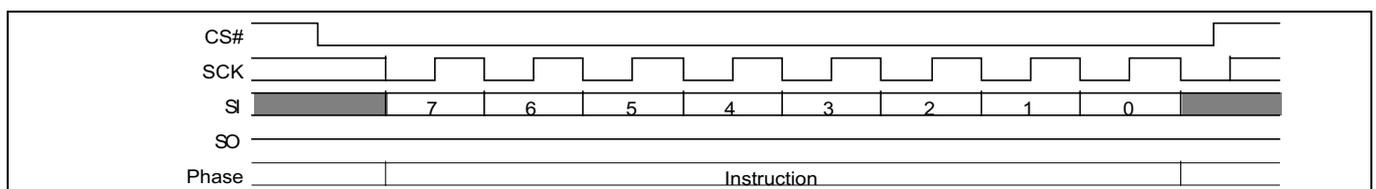
**Figure 101 Erase resume (ERRS 7Ah) command sequence**
