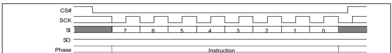
**Figure 57 Clear status register (CLSR 30h) command sequence**
