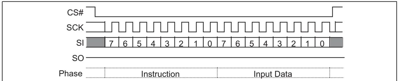
**Figure 64 Write VDLR (WVDLR 4Ah) command sequence**
