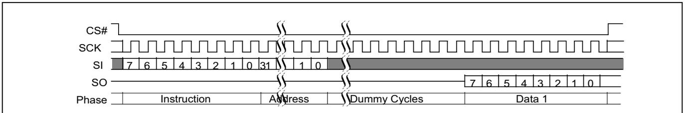
**Figure 11 Single bit wide I/O command with latency**
