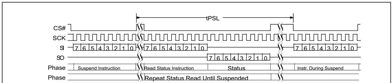
**Figure 96 Program suspend (PGSP 85h) command sequence**
