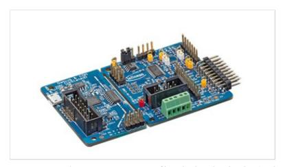
Discover more about our **EVAL-M1-1302** (/cms/en/product/evaluation-boards/eval-m1-1302/) motor control board powered by **XMC 1302** (/cms/en/product/channel.html?channel=db3a30433c1a8752013c1aa35a6a0029). It includes an isolated J-Link interface by Segger. The Hardware is prepared to use HALL- or latest innovation of 3D Magnetic Sensor. A complete development suite consisting of DAVE and  $\mu$ C-Probe is provided.
