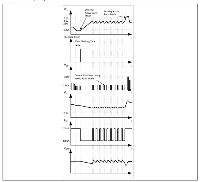
Figure 25 **Signals in Active Burst Mode**
