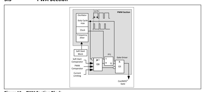
Figure 15 PWM Section Block
