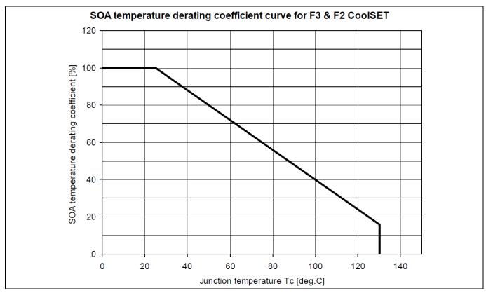
Figure 29 SOA temperature derating coefficient curve
