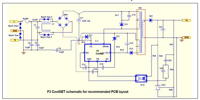
Figure 36 Schematic for recommended PCB layout
