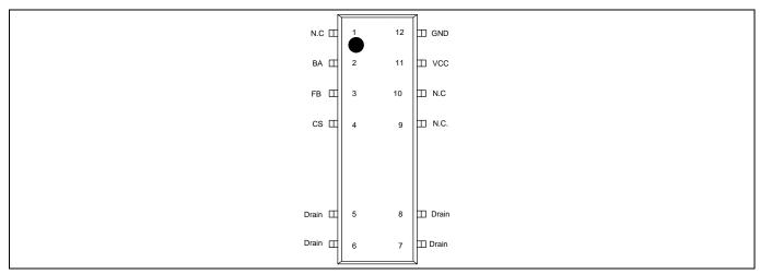
Figure 2 Pin configuration PG-DSO-12(top view)
