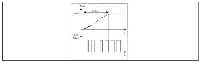
Figure 13 **Gate drive signal under Soft-Start Phase**
