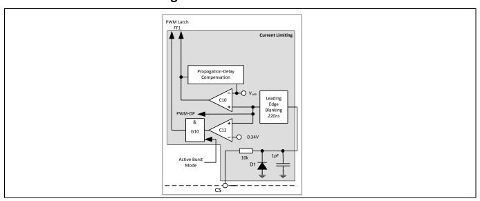
Figure 18 Current Limiting Block
