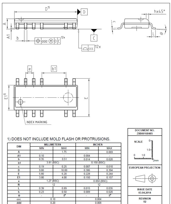
Figure 34 PG-DSO-12 (Pb-free lead plating Plastic Dual-in-Line Outline)
