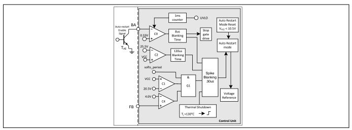
Figure 27 Over load, open loop protection
