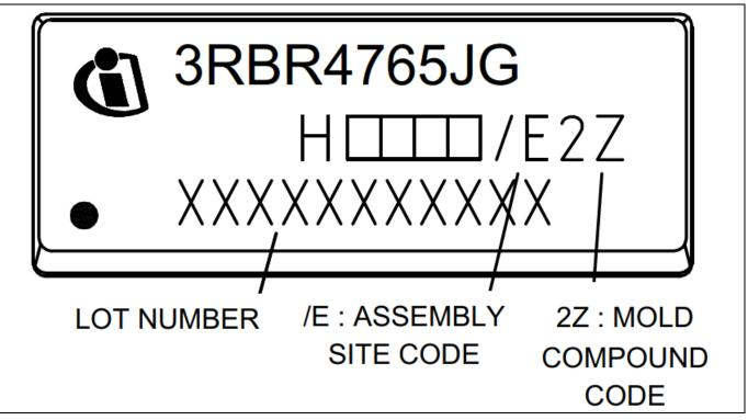
Figure 35 Marking for ICE3RBR4765JG
