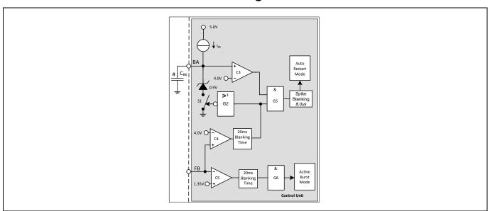
Figure 23 Basic and Extendable Blanking Mode
