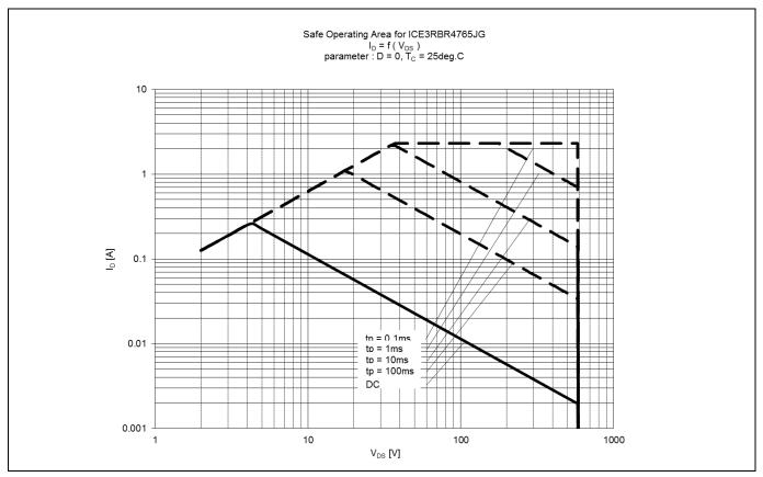
Figure 28 Safe Operating Area (SOA) curve for ICE3RBR4765JG
