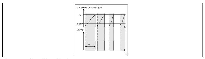
Figure 6 Pulse Width Modulation
