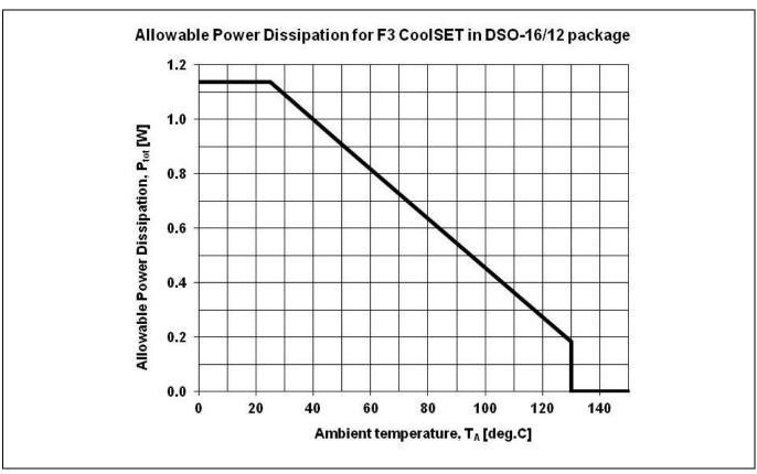
Figure 30 Power dissipation; P<sub>tot</sub>=f(T<sub>a</sub>)
