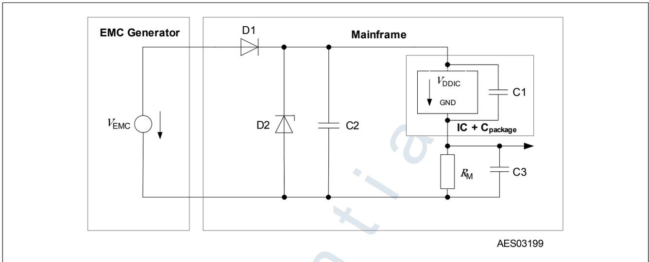
Figure 9 EMC test circuit
