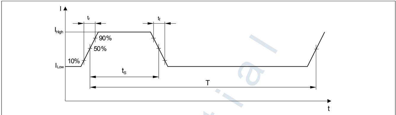
Figure 8 Definition of Rise and Fall time; Duty Cycle =  $(t_s / T) \times 100\%$
