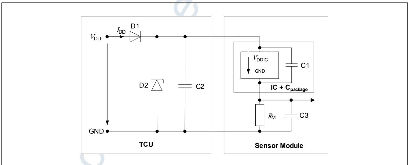
Figure 10 Application circuit
