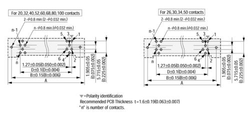
TS-2051-B Sheet 2 of 3 .050" Straight and Right Angle Plug, with Power Ground Pin
