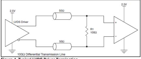
Figure 4. Typical LVDS Driver Termination
