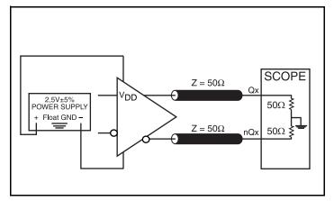
LVDS Output Load AC Test Circuit
