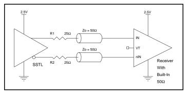
Figure 2B. IN/nIN Input with Built-In 50 $\Omega$  Driven by an SSTL Driver
