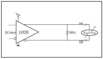
**Differential Output Voltage Setup**
