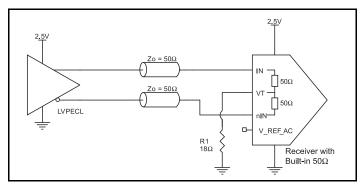
Figure 2D. IN/nIN Input with Built-In 50 $\Omega$  Driven by an LVPECL Driver
