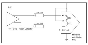
Figure 2C. IN/nIN Input with Built-In 50 $\Omega$  Driven by a CML Driver
