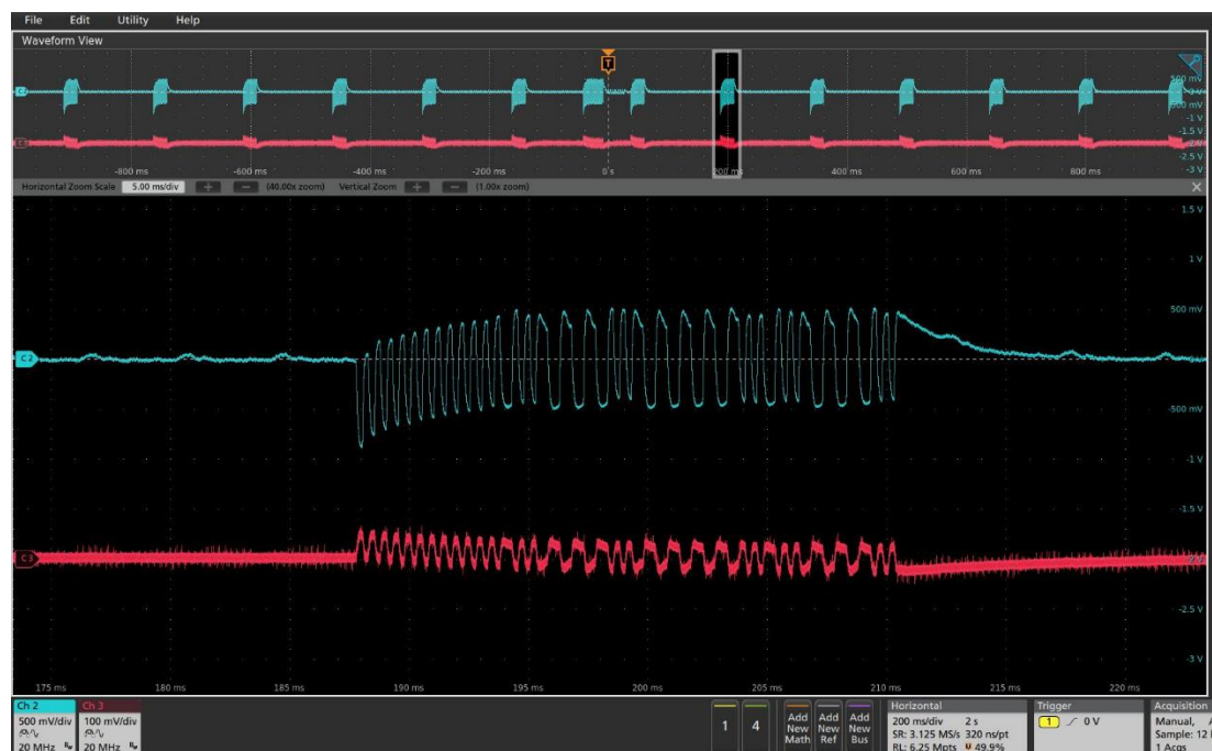
Figure 7. Voltage and Current Signal for Demodulation: Ch2 = VSNS, Ch3 = ISNS_IN
