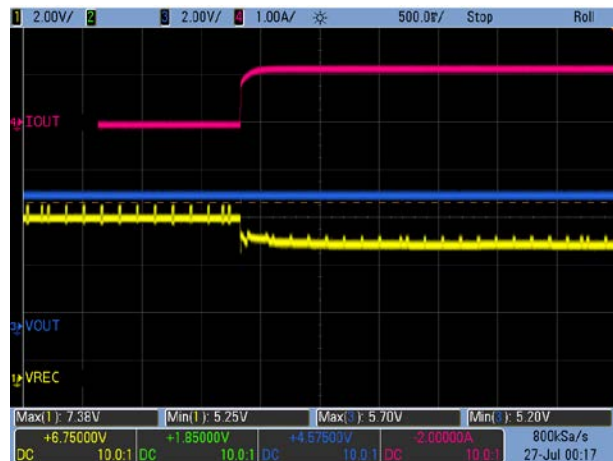
Figure 11. Load Transient: V_{OUT} = 5V , 0A \rightarrow 1.2A
