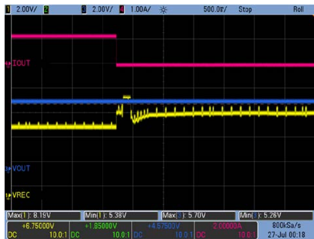
Figure 12. Load Transient: V OUT = 5V, 1.2A → 0A
