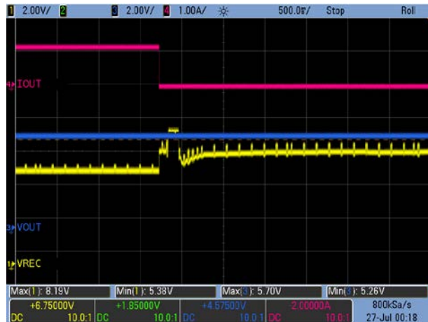
Figure 12. Load Transient: V_{OUT} = 5V , 1.2A \rightarrow 0A
