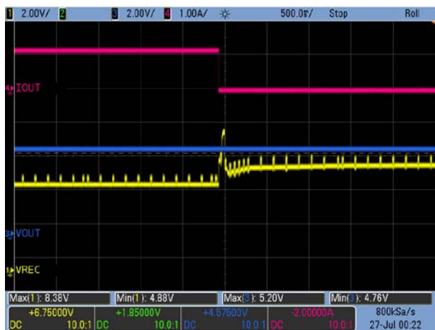
Figure 12. Load Transient: V OUT = 5V, 1.2A → 0A
