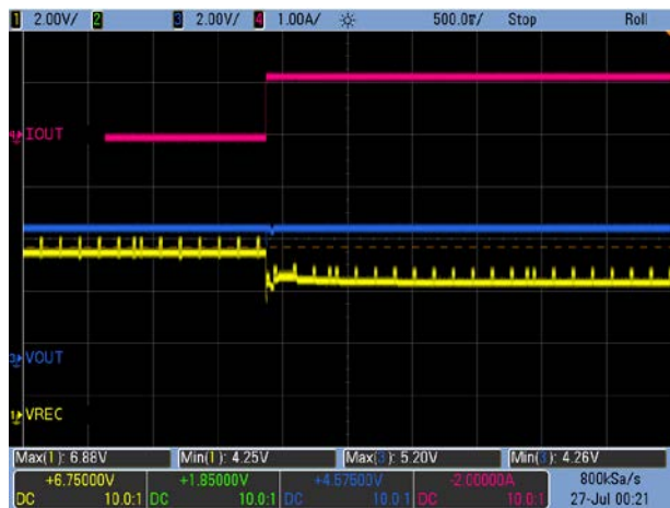
Figure 11. Load Transient: V OUT = 5V, 0A → 1.2A
