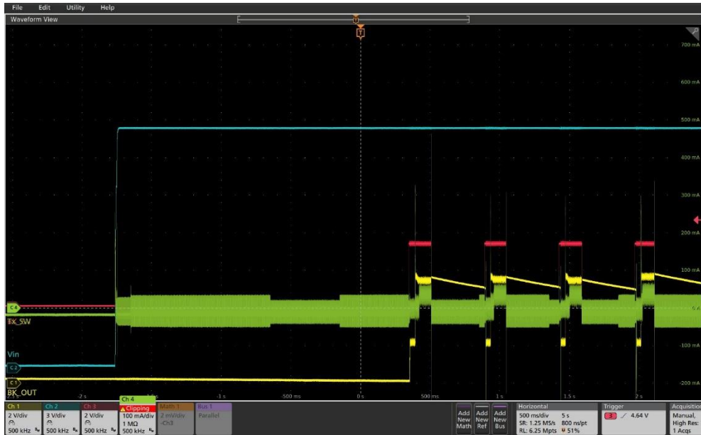
Figure 13. 19V Fixed Voltage Adaptor Start-up: Ch1 = VBRIDGE, Ch2 = V_{in} , Ch3 = GPIO_B4, Ch4 = i_{in}
