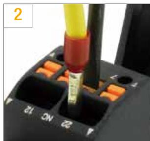
While holding down the pusher, remove the wire.
