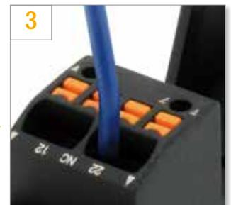
Release the flat-blade screwdriver. Connection is completed. Pull lightly to make sure it is firmly in place.
