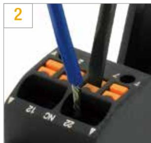
While holding down the pusher, insert the wire to the back of the wire port.
