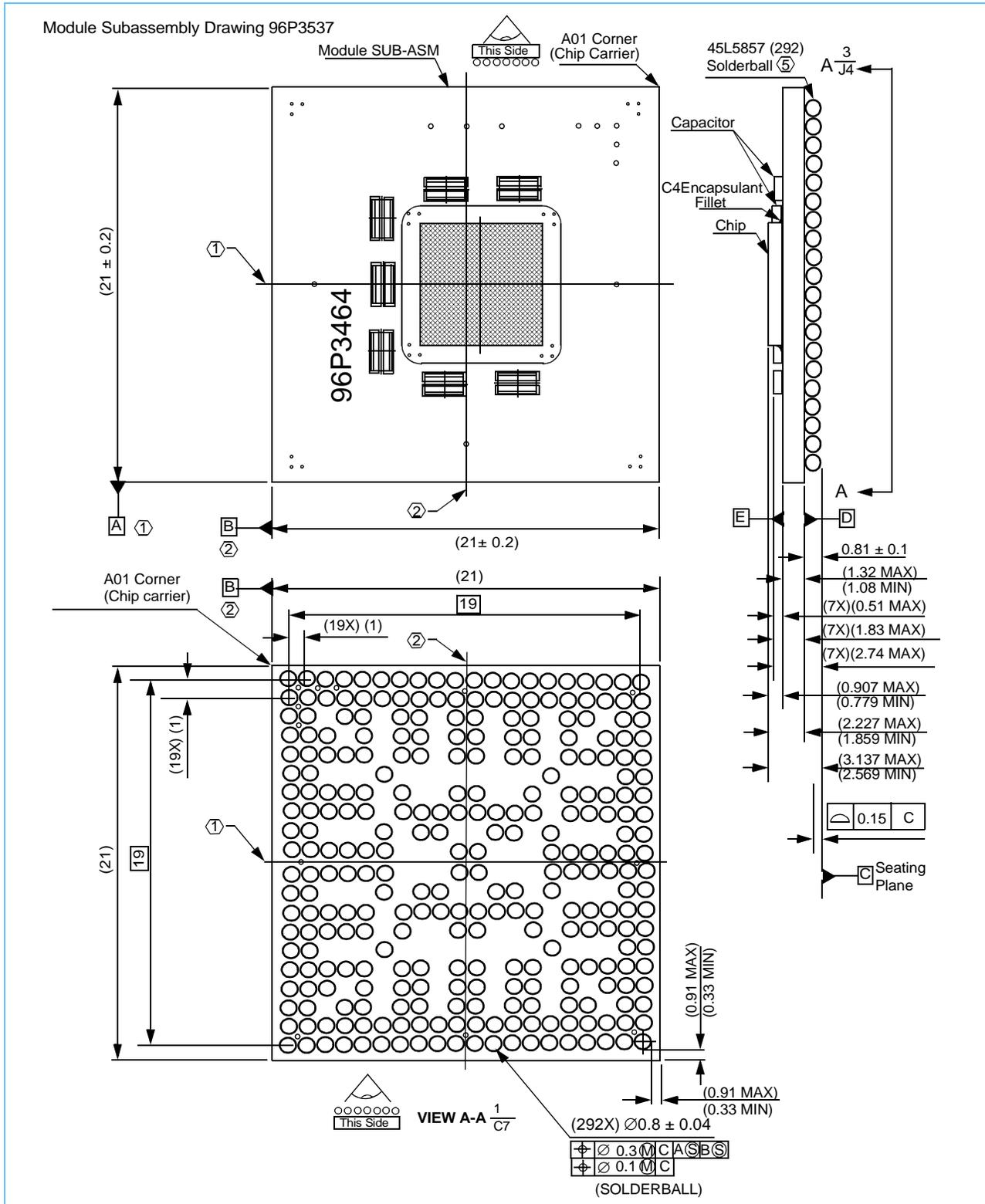
*Figure 4-1. Mechanical Dimensions, Standard (Leaded) Package(Continued)*
