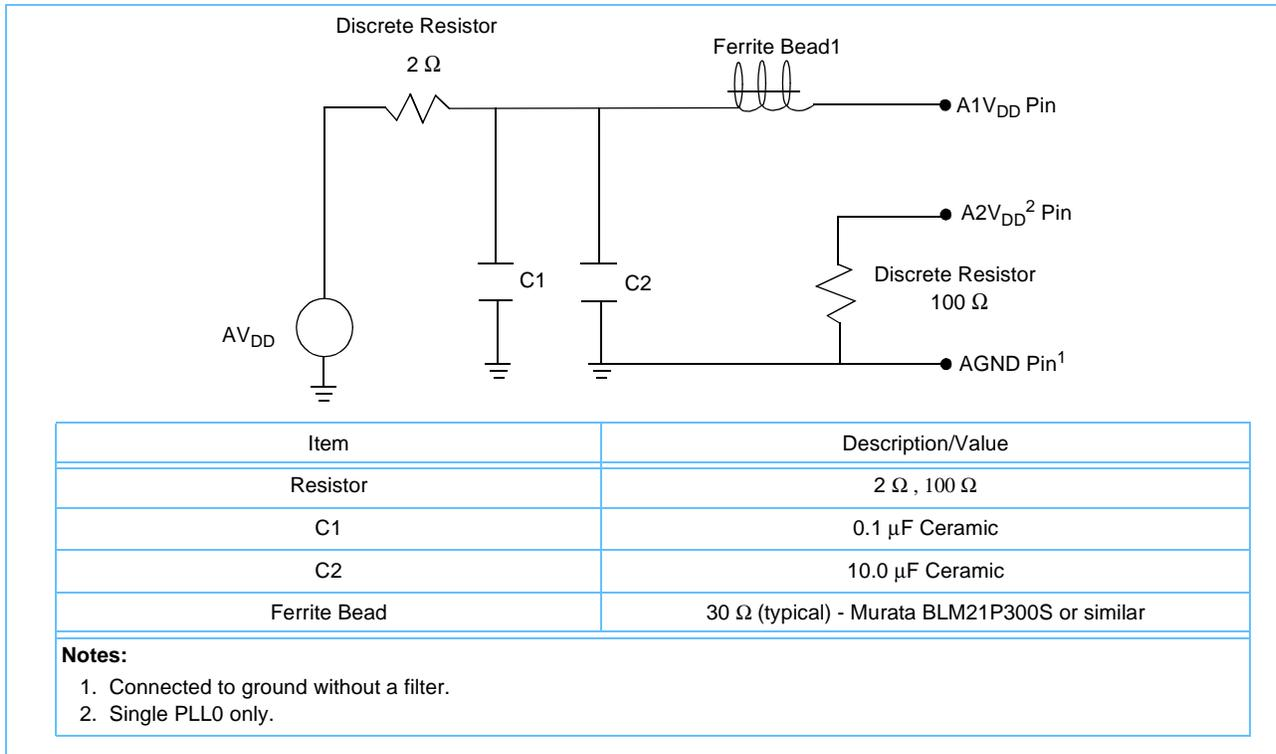
**Figure 5-2. PLL Power Supply Filter Circuit with Two AV<sub>DD</sub> Pins and One Ferrite Bead (Optional)**
