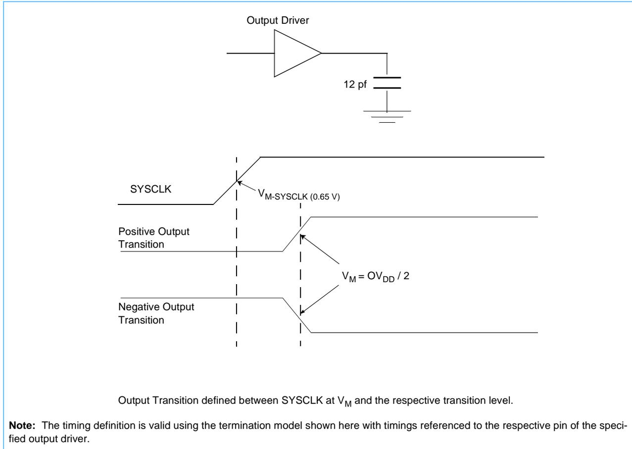
Figure 3-7. Output Timing Diagram for IBM PowerPC 750GX RISC Microprocessor
