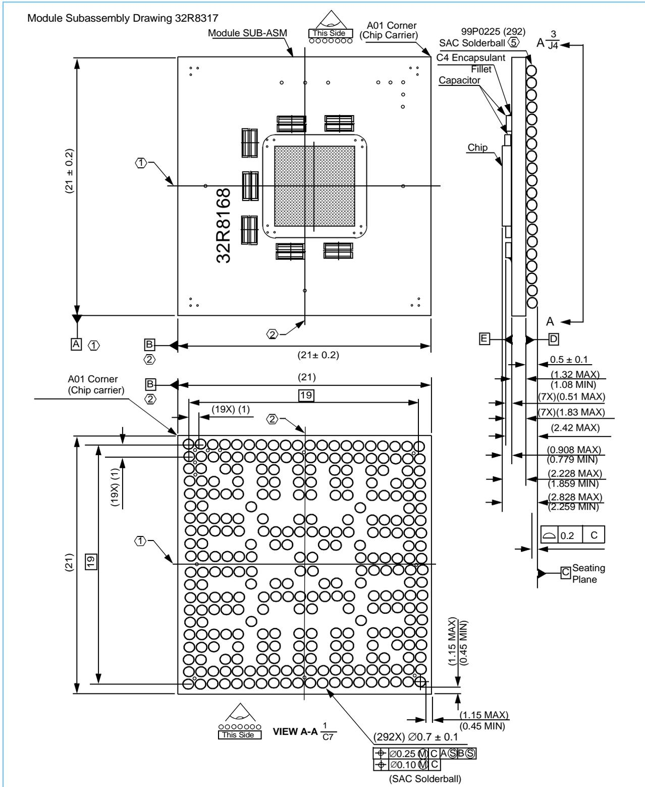
*Figure 4-2. Mechanical Dimensions, ROHS-Compatible Package (Continued)*
