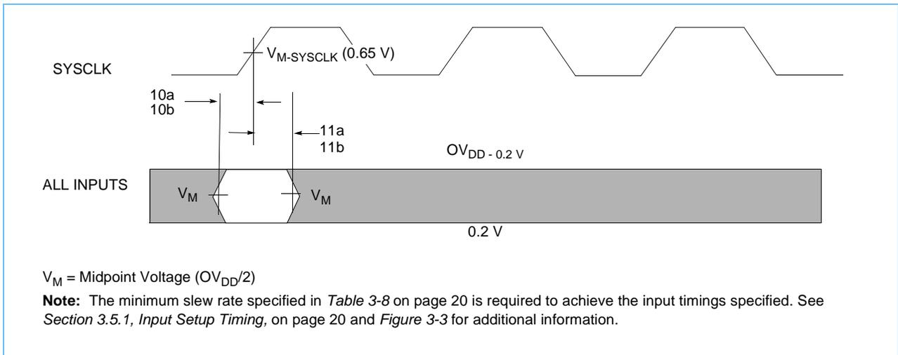
Figure 3-5 provides the mode select input timing diagram for the 750GX.
