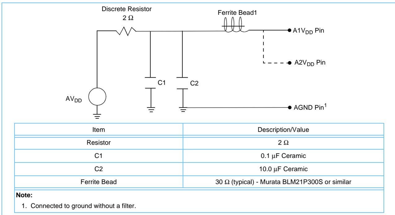
Figure 5-3. Dual PLL Power Supply Filter Circuits (Recommended if Dual-PLL is Enabled)<sup>1</sup>
