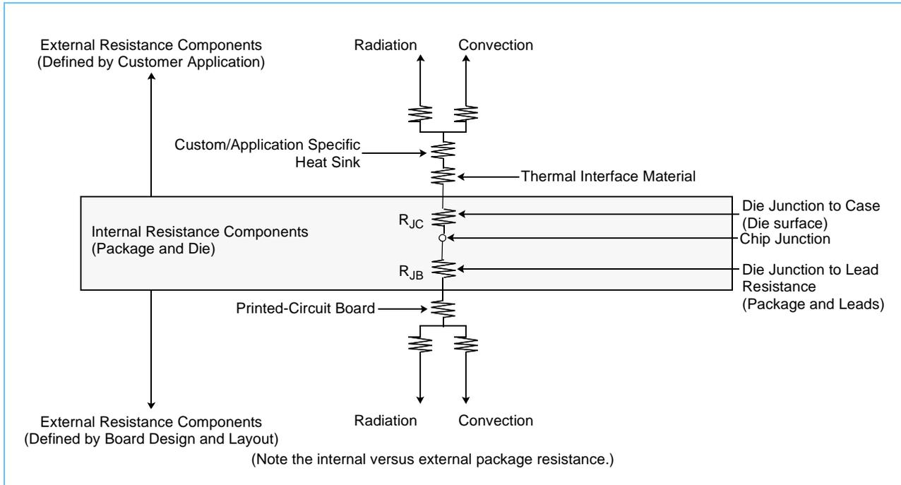
Heat generated on the active side (ball) of the chip is conducted through the silicon, then through the heat-sink attach material (or thermal interface material), and finally to the heat sink; where it is removed by forced-air convection. Since the silicon thermal resistance is quite small, for a first-order analysis, the temperature drop in the silicon may be neglected. Thus, the heat sink attach material and the heat-sink conduction/convective thermal resistances are the dominant terms.
