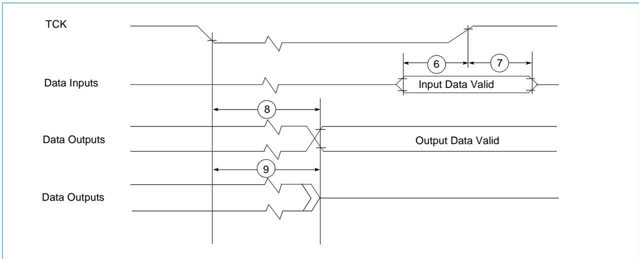
Figure 3-11 provides the test access port timing diagram.
