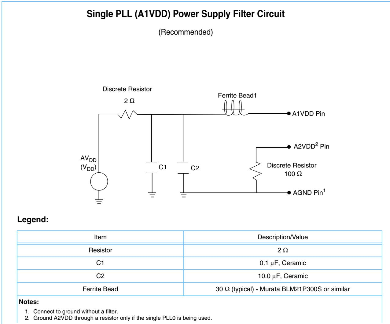
Figure 5-2. PLL Power Supply Filter Circuit with Two AV<sub>DD</sub> Pins and One Ferrite
