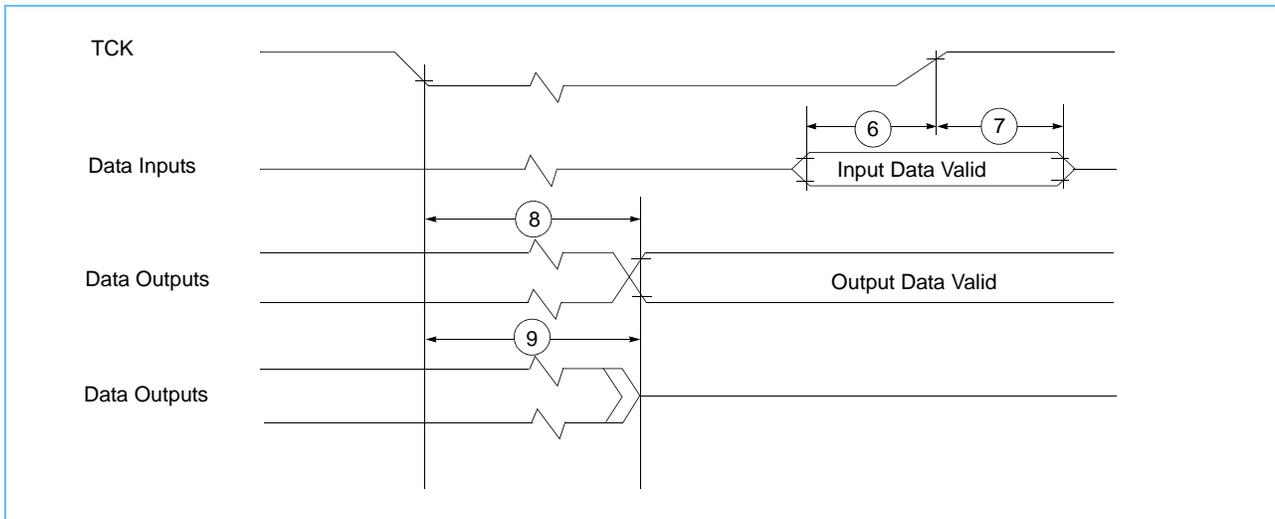
Figure 3-10. Test Access Port Timing Diagram
