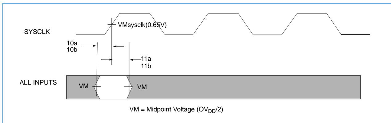
Figure 3-4 provides the mode select input timing diagram for the 750FL microprocessor.
