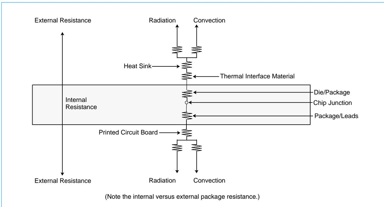
Heat generated on the active side of the chip is conducted through the silicon, then through the heat sink attach material (or thermal interface material), and finally to the heat sink; where it is removed by forced-air convection. Because the silicon thermal resistance is quite small, for a first-order analysis, the temperature drop in the silicon can be neglected. Thus, the heat sink attach material and the heat sink conduction/convection thermal resistances are the dominant terms.
