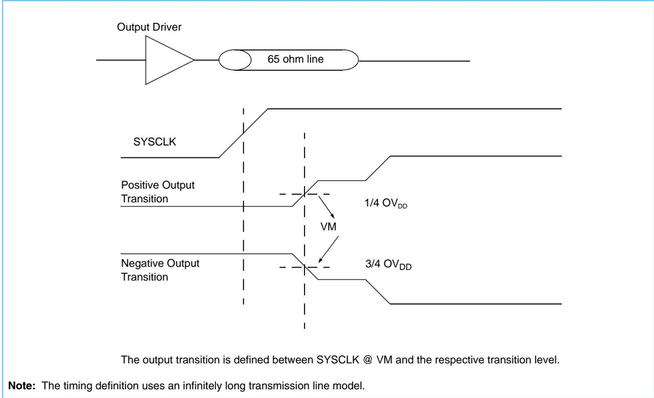
Figure 3-6. Output Timing Diagram for PowerPC 750FL RISC Microprocessor
