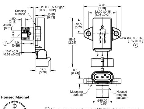
1 Non-magnetic, stainless steel M3 X 0.5 plain cup point set screws, torque is 0,5 N m to 0,6 N m [4.42 in-lb to 5.31 in-lb]
