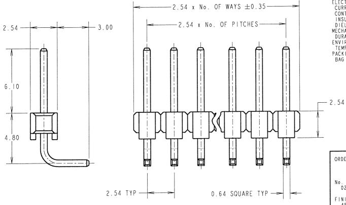
SPECIFICATION: MATERIAL: MOULDING = HIGH TEMP NYLON 6T UL94V-0, BLACK PINS = BRASS FINISH: PINS: 45 = GOLD 46 = 100% TIN OVER NICKEL ELECTRICAL: CURRENT RATING = 3A MAX CONTACT RESISTANCE = 25 m $\Omega$  MAX (GOLD), 30 m $\Omega$  MAX (TIN) INSULATION RESISTANCE = 1,000 M $\Omega$  MIN DIELECTRIC STRENGTH = 750V AC/DC MECHANICAL: DURABILITY = 300 OPERATIONS (GOLD), 50 OPERATIONS (TIN) ENVIRONMENTAL: TEMPERATURE RANGE = -40°C TO +105°C PACKING: BAG
