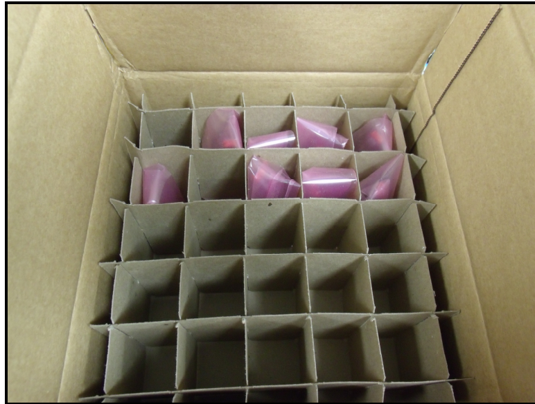
Figure 8 – DUT Packaging after Transit Drop
