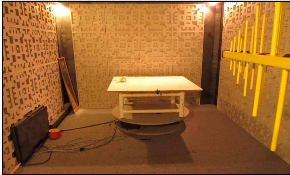
Figure 4 – DUT under Radiated Emissions Test
