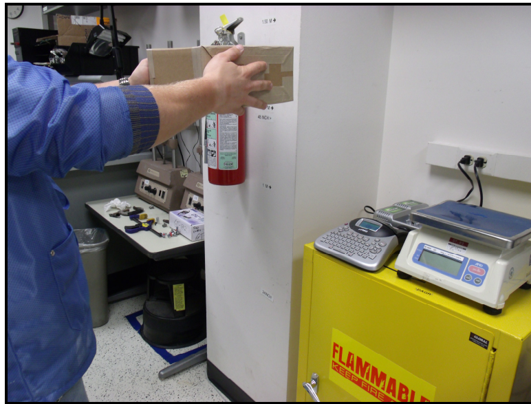
Figure 6 – Transit Drop Set Up
