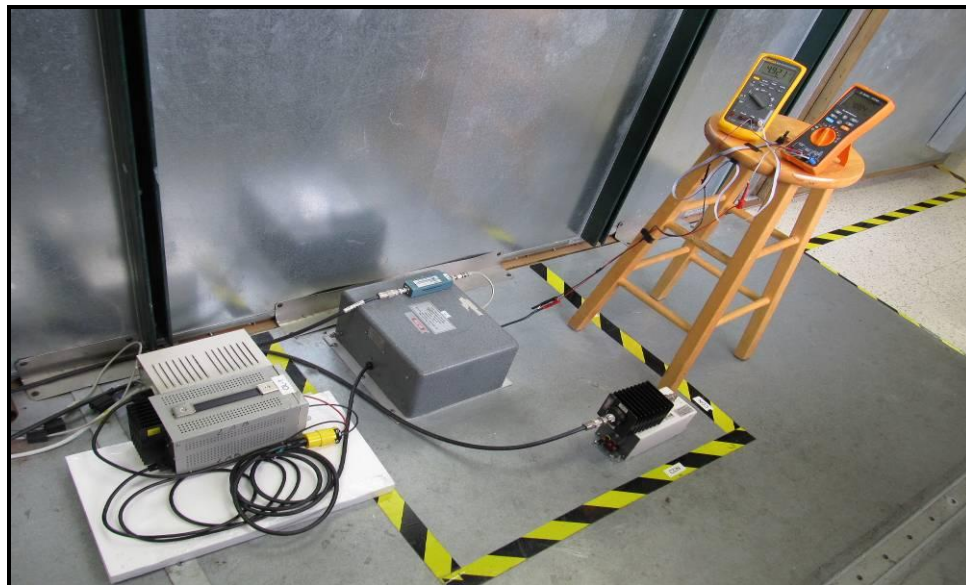
Figure 7 - Conducted Emissions Test Setup
