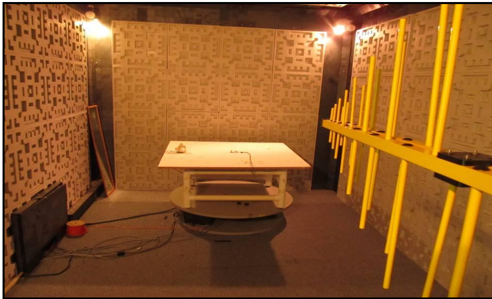
Figure 1 - Radiated Immunity Test Setup
