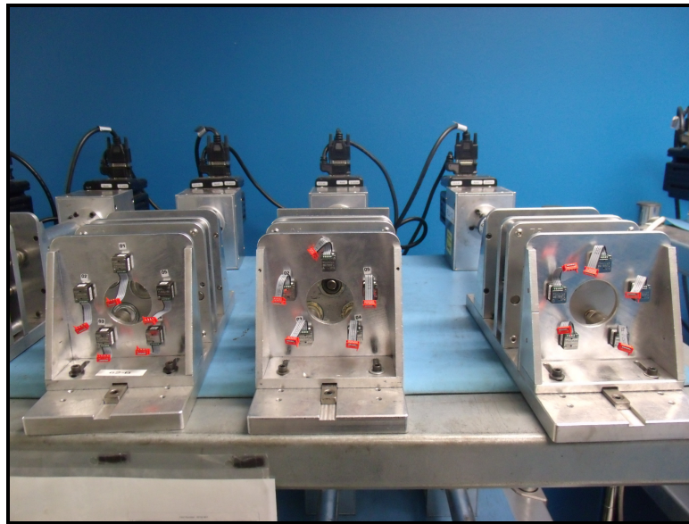
Figure 19 – Rotational Life Test Setup
