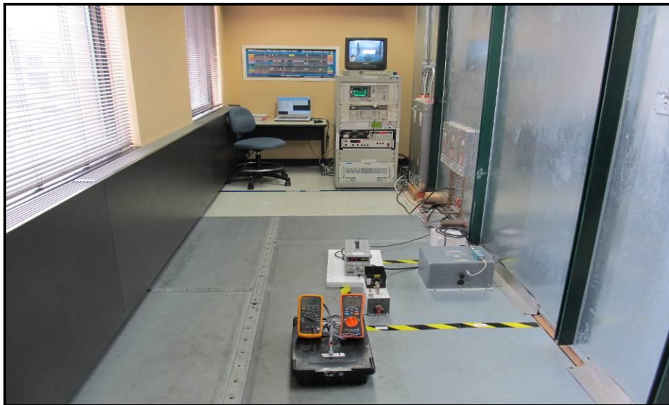
Figure 6 – Conducted Immunity test setup
