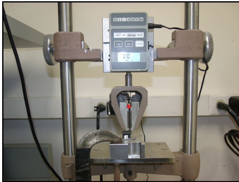
Figure 4– Cable Strength Setup
