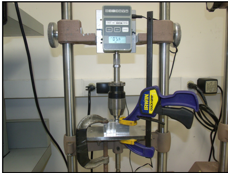
Figure 3– Pull Out Force Setup
