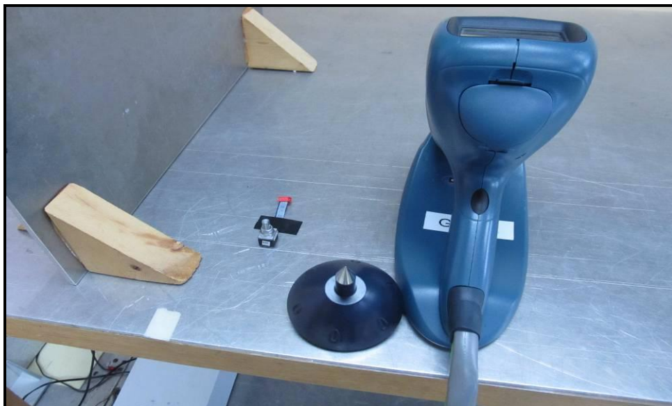
Figure 10 – Electrostatic Discharge Test Setup (Un-Powered)
