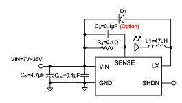
\*The PCB layout of G2610 must be carefully designed, otherwise the SENSE pin would be disturbed. An optioned 0.1µF decoupling capacitor(Cs) between VIN and SENSE is suggested, please place it as closely to VIN and SENSE as possible.
