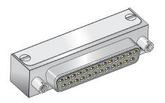
Low profile right angle PC tail HiPer-D® socket connectors feature rugged machined aluminum shell and stainless steel cover for improved EMI protection. Contacts are non-removable size, #20 or #22. Intermateable with standard M24308-type D-Subminiature connectors, the HiPer-D® features epoxy potting for environmental sealing. Threaded holes on the rear of the connector allow attachment to circuit board. Glass-reinforced thermoset epoxy insulators. 1000 VAC, 5 Amps (#22) or 7.5 Amps (#20).
