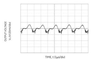
Figure 15. Typical output ripple and noise (V<sub>IN</sub> = 12V, Io =  $I_{O,mox}$ ).
