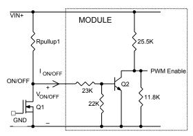
Figure 43. Circuit configuration for using negative On/Off logic.
