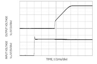
Figure 29. Typical Start-up Using On/Off Voltage ( $I_0 = I_{0,max}$ ).
