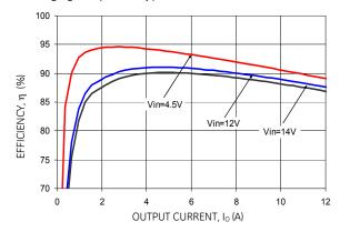
Figure 13. Converter Efficiency versus Output Current.
