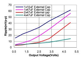
Figure 41. Output ripple voltage for various output voltages with external 1x10  $\mu$ F, 1x47  $\mu$ F, 2x47  $\mu$ F or 4x47  $\mu$ F ceramic capacitors at the output (12A load). Input voltage is 12V.
