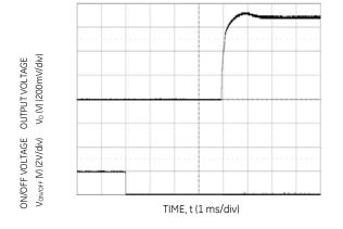
Figure 5. Typical Start-up Using On/Off Voltage ( $I_0 = I_{0,max}$ ).
