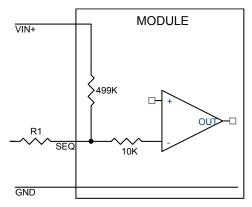
Figure 47. Circuit showing connection of the sequencing signal to the SEO pin.
