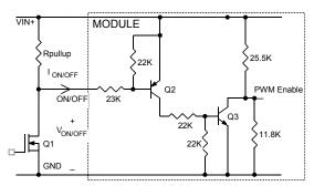
Figure 42. Circuit configuration for using positive On/Off logic.
