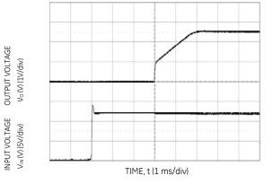
Figure 23. Typical Start-up Using On/Off Voltage ( $I_0 = I_{0,max}$ ).
