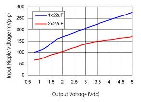
Figure 40. Input ripple voltage for various output voltages with 1x22  $\mu$ F or 2x22  $\mu$ F ceramic capacitors at the input (12A load). Input voltage is 12V.
