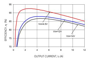
Figure 7. Converter Efficiency versus Output Current.
