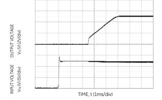
Figure 33. Typical Start-up Using On/Off Voltage ( $I_0 = I_{0,max}$ ).
