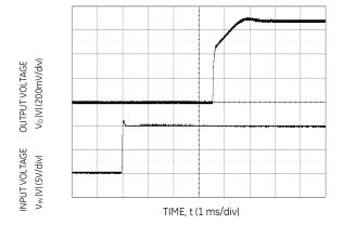
Figure 6. Typical Start-up Using Input Voltage ( $V_{IN} = 10V$ ,  $I_0 = I_{0,max}$ ).
