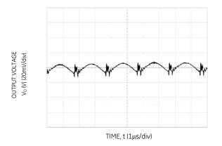
Figure 3. Typical output ripple and noise ( $V_{IN} = 12V$ ,  $I_0 = I_{O,max}$ ).
