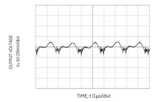
Figure 9. Typical output ripple and noise ( $V_{IN} = 12V$ ,  $I_0 = I_{O,max}$ ).
