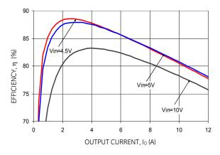
Figure 1. Converter Efficiency versus Output Current.
