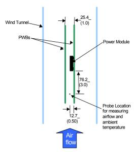
Figure 49. Thermal Test Setup.
