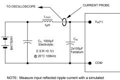
NOTE: Measure input reflected ripple current with a simulated source inductance (L<sub>TEST</sub>) of 1µH. Capacitor C<sub>S</sub> offsets possible battery impedance. Measure current as shown above
