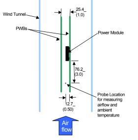
Figure 49. Thermal Test Setup.
