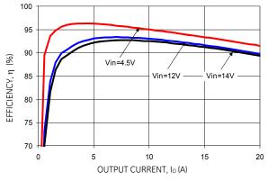
Figure 25. Converter Efficiency versus Output Current.
