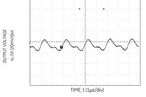
Figure 21. Typical output ripple and noise (V  $_{\rm IN}$  = 12V,  $I_{\rm o}$  =  $I_{o,max}$ ).
