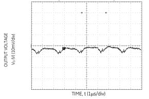
Figure 3. Typical output ripple and noise ( $V_{IN} = 12V$ ,  $I_0 = I_{0,max}$ ).
