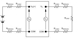
NOTE: All voltage measurements to be taken at the module terminals, as shown above. If sockets are used then Kelvin connections are required at the module terminals to avoid measurement errors due to socket contact resistance.
