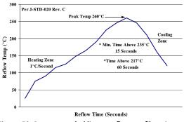
Figure 50. Recommended linear reflow profile using Sn/Ag/Cu solder.
