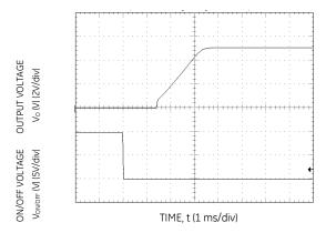
Figure 33. Typical Start-up Using On/Off Voltage ( $I_0 = I_{0,max}$ ).
