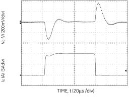
Figure 28. Transient Response to Dynamic Load Change from 0% 50% to 0%.
