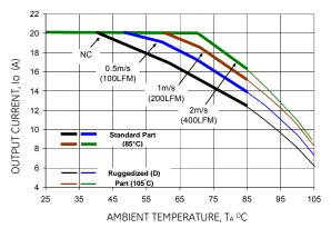
Figure 20. Derating Output Current versus Ambient Temperature and Airflow. Ruggedized part is discontinued
