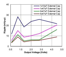
Figure 41. Output ripple voltage for various output voltages with external 1x10  $\mu F,$  1x47  $\mu F,$  2x47  $\mu F$  or 4x47  $\mu F$  ceramic capacitors at the output (20A load). Input voltage is 12V.
