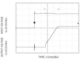
Figure 30. Typical Start-up Using Input Voltage (ViN = 12V,  $I_{0}$  =  $I_{0,max}$ ).
